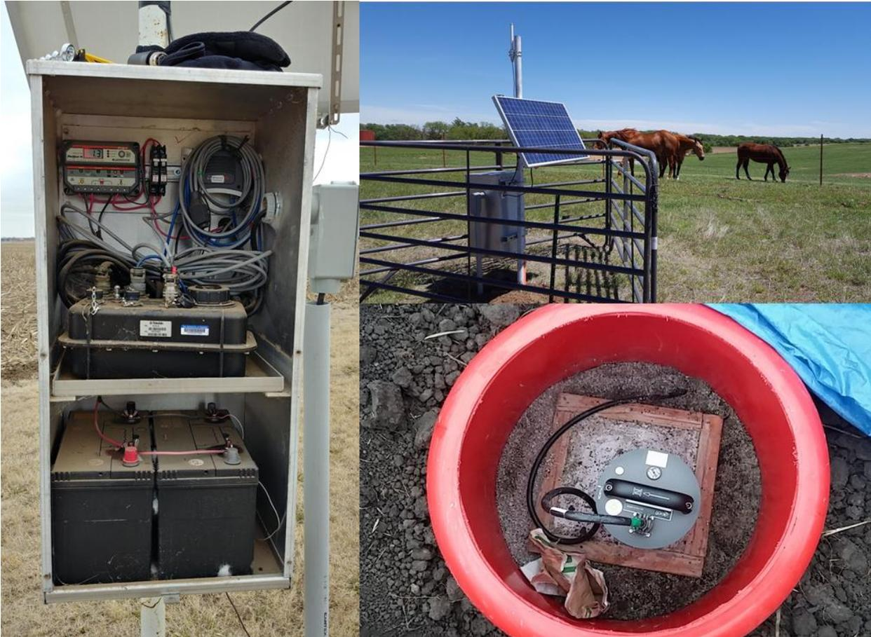
Figure 3-4 – Typical earthquake seismic station (top right), inverted bucket housing seismometer (bottom right) and equipment box attached to the solar panel pole (left).
