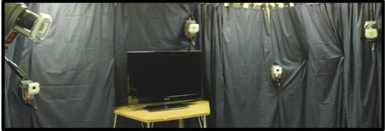
Figure 2b: Infrared motion capture suite with camera array aimed at infant's 3D work space.
