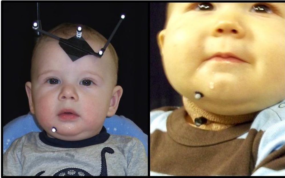
Figure 1: Head block array and jaw marker (left); Jaw marker and laryngeal accelerometer (right)
