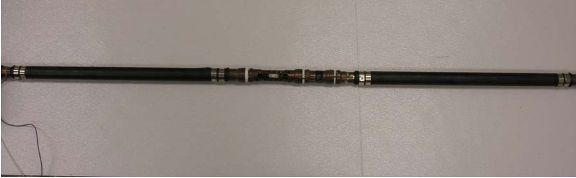
Figure 8 – Pumped hydraulic source assembly consisting of an injection interval straddled between two packers.
