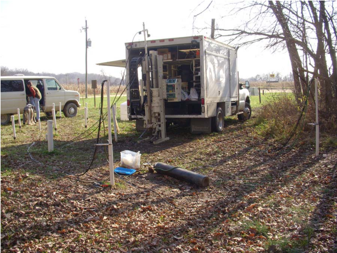
Figure 11 – Pneumatic injection apparatus for the CPT with Geoprobe. The receivers are in HT-3 (left) and HT-2 (right) located in the foreground of the picture.
