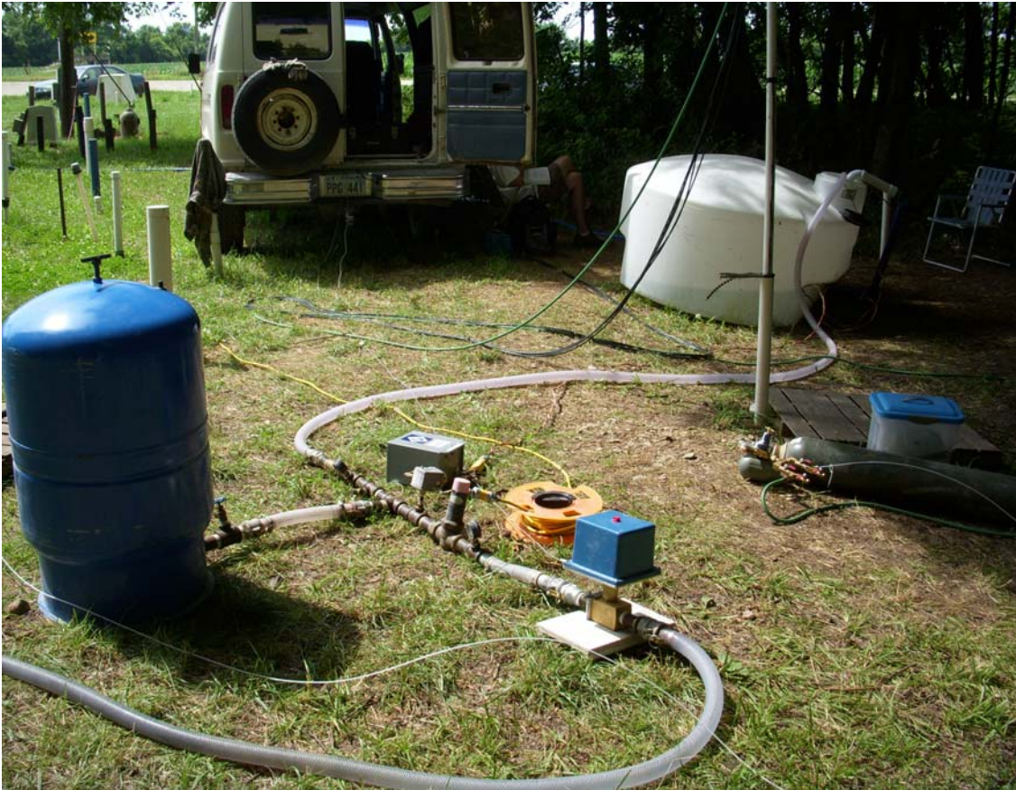
Figure 9 – Pumped hydraulic injection apparatus for the CPT.
