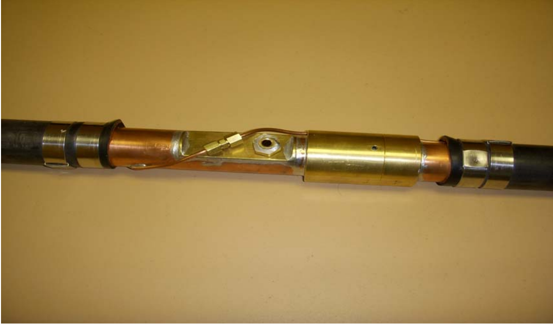
Figure 6 – Transducer port located between the straddle packers of the new receiver.
