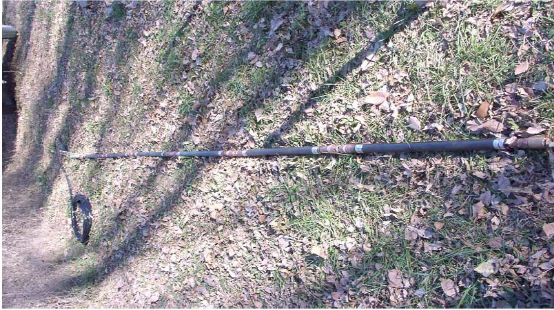
Figure 5 – A 5-channel receiver consisting of 5 transducers on 0.914 m (3 ft) centers isolated by 6 packers. Figure modified from Wachter (2008).
