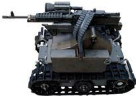
Figure 2: The S.W.O.R.D.S. robot - uses tracks for locomotion requiring a semi-continuous path. [1]
