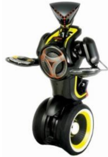
Figure 1: The A.M.P. robot - uses wheels for locomotion requiring a continuously smooth path [14]
