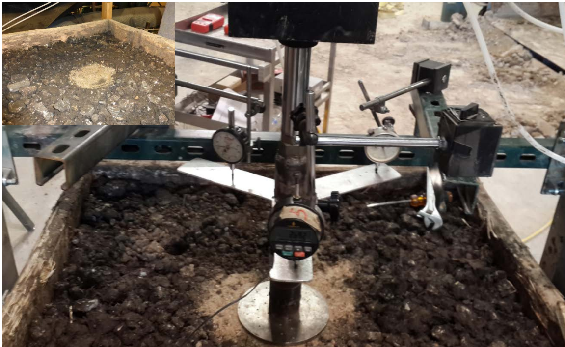
Figure 4-19 Plate Loading Test Set up
