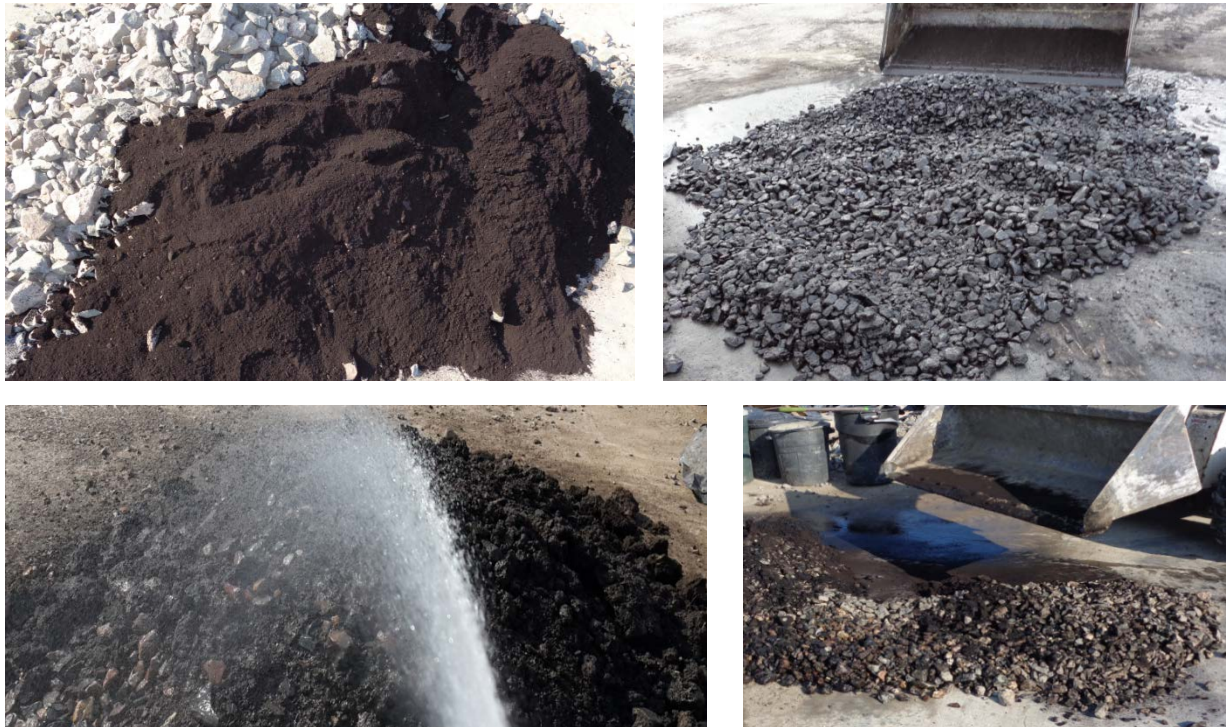
Figure 4-2 Mixing Procedure Started from Top Left Corner Running Counterclockwise The close views of the mixed ballast with different fouling agents are shown in Figure 4.3.
