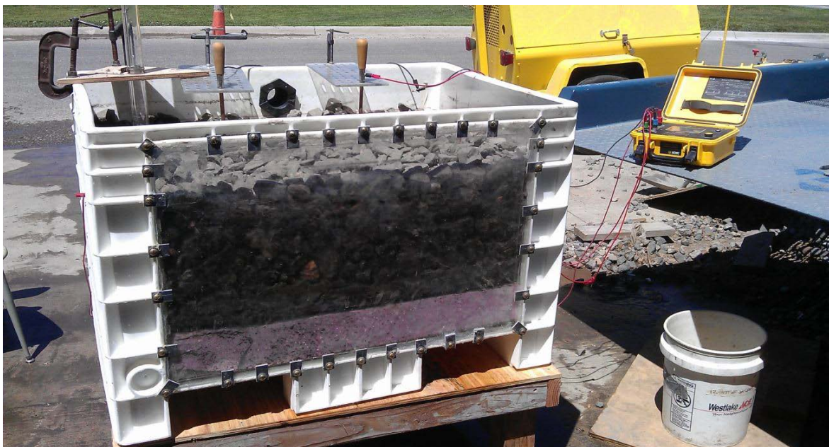
Figure 2-5 Resistivity Measurement Test Set up by Wenner 4 Point Method (Rahman, 2014)
