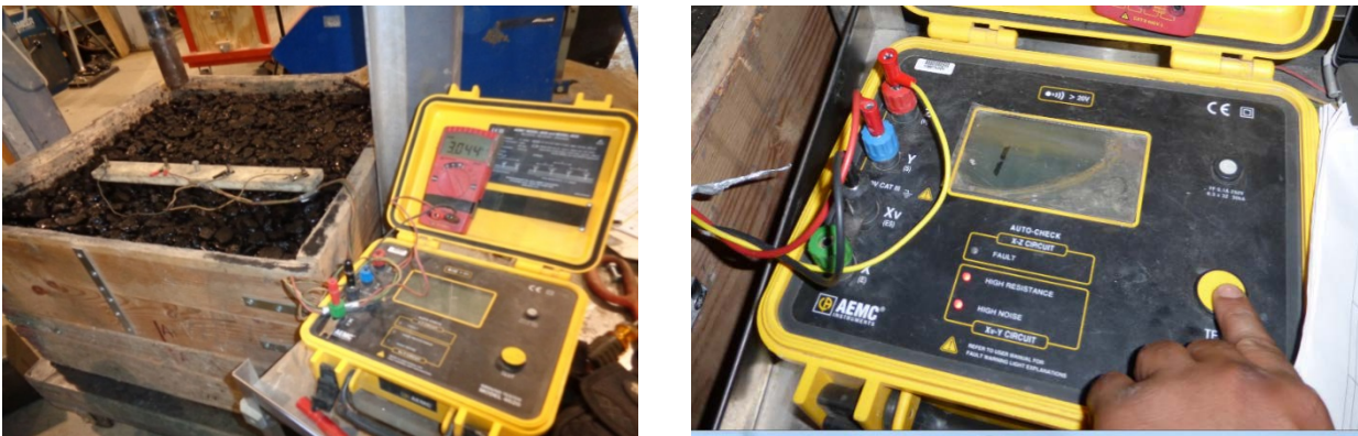
Figure 4-11 Resistance Measurement by Wenner Four Point Method with AMCE Tester
