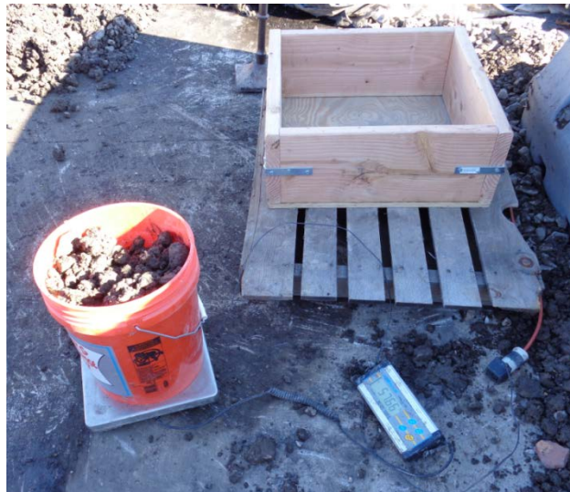
Figure 5-3 Dry Density Determination from Small Box Test
