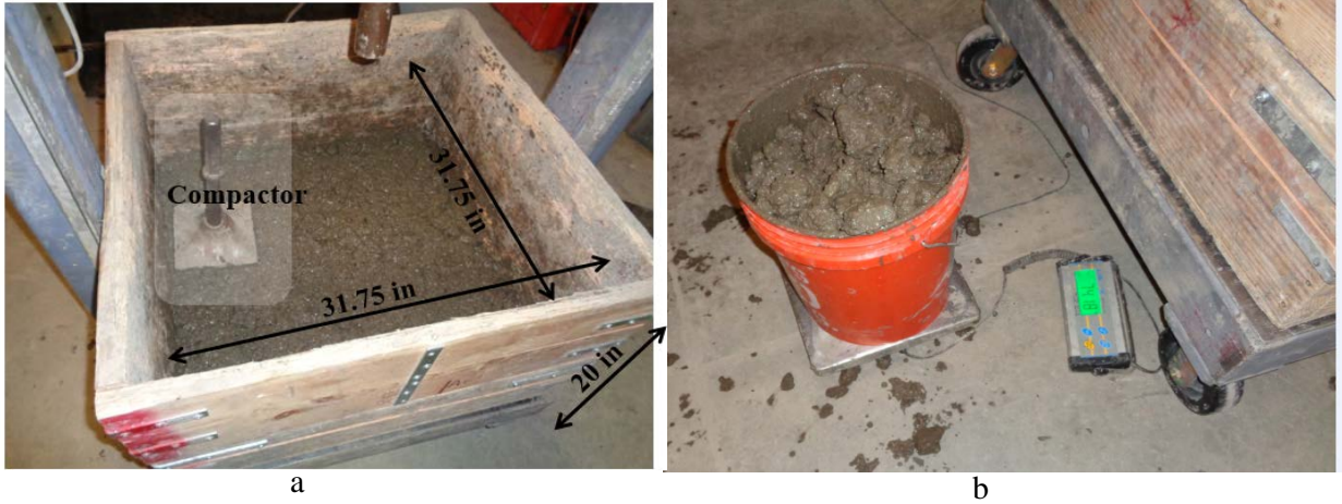
Figure 4-5 Filling Procedure (a) Compaction of Sample (b) Weighing before Pouring to Box
