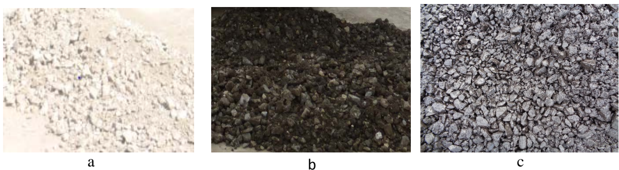
Figure 4-3 Artificially Fouled Ballast Ready to Go into Test Box (a) Crushed Stone Fouled (b) Subgrade Soil Fouled (c) Coal Dust Fouled
