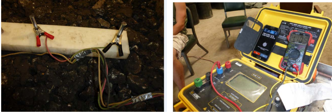
Figure 4-12 Fouled Ballast Resistance Measurement by Single Probe Method
