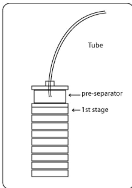
**Figure 2.1** A diagram of cascade impactor with a tube.
