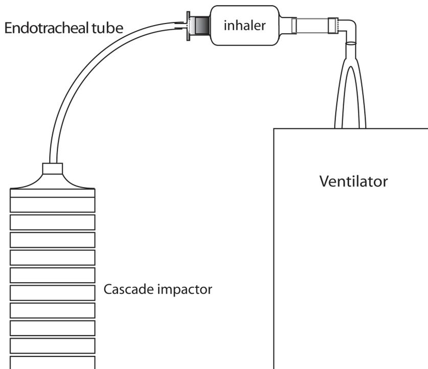
**Figure 3.2** A schematic diagram of the DPI connected between the ventilator and the cascade impactor.
