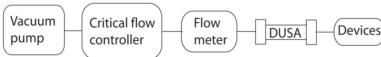
**Figure 3.3** Experimental set-up for pressure drop measurement.
