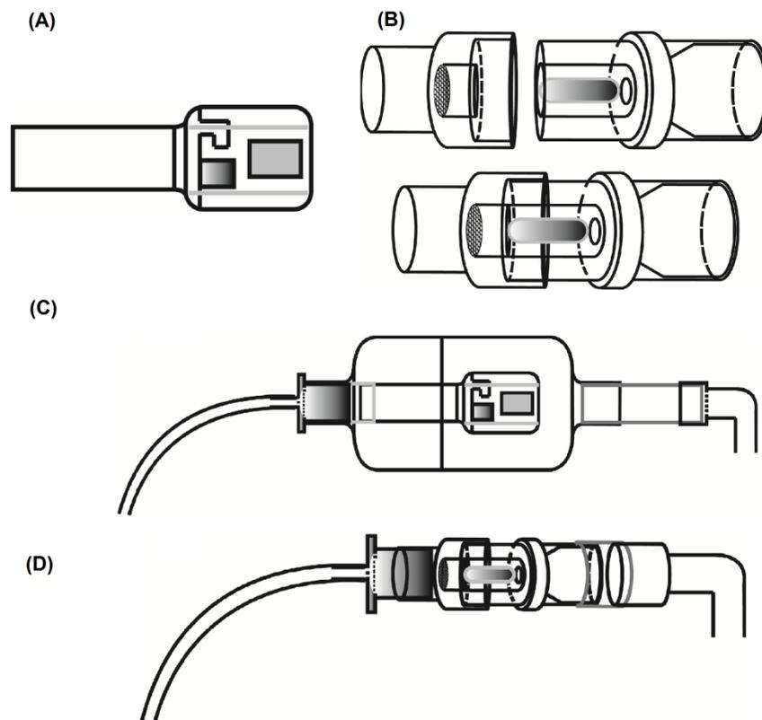
**Figure 3.8** Schematic diagrams of (A) the Monodose<sup>®</sup> inhaler, (B) the novel device, (C) the Monodose<sup>®</sup> inhaler connected to the mechanical ventilator circuit, and (D) the novel device connected to the mechanical ventilator circuit.
