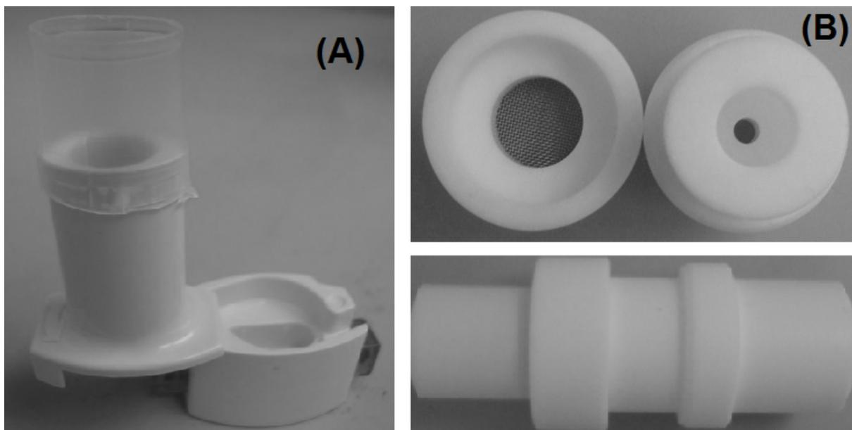
**Figure 3.1** Photographs of (A) the modified Monodose<sup>®</sup> inhaler and (B) the novel device.
