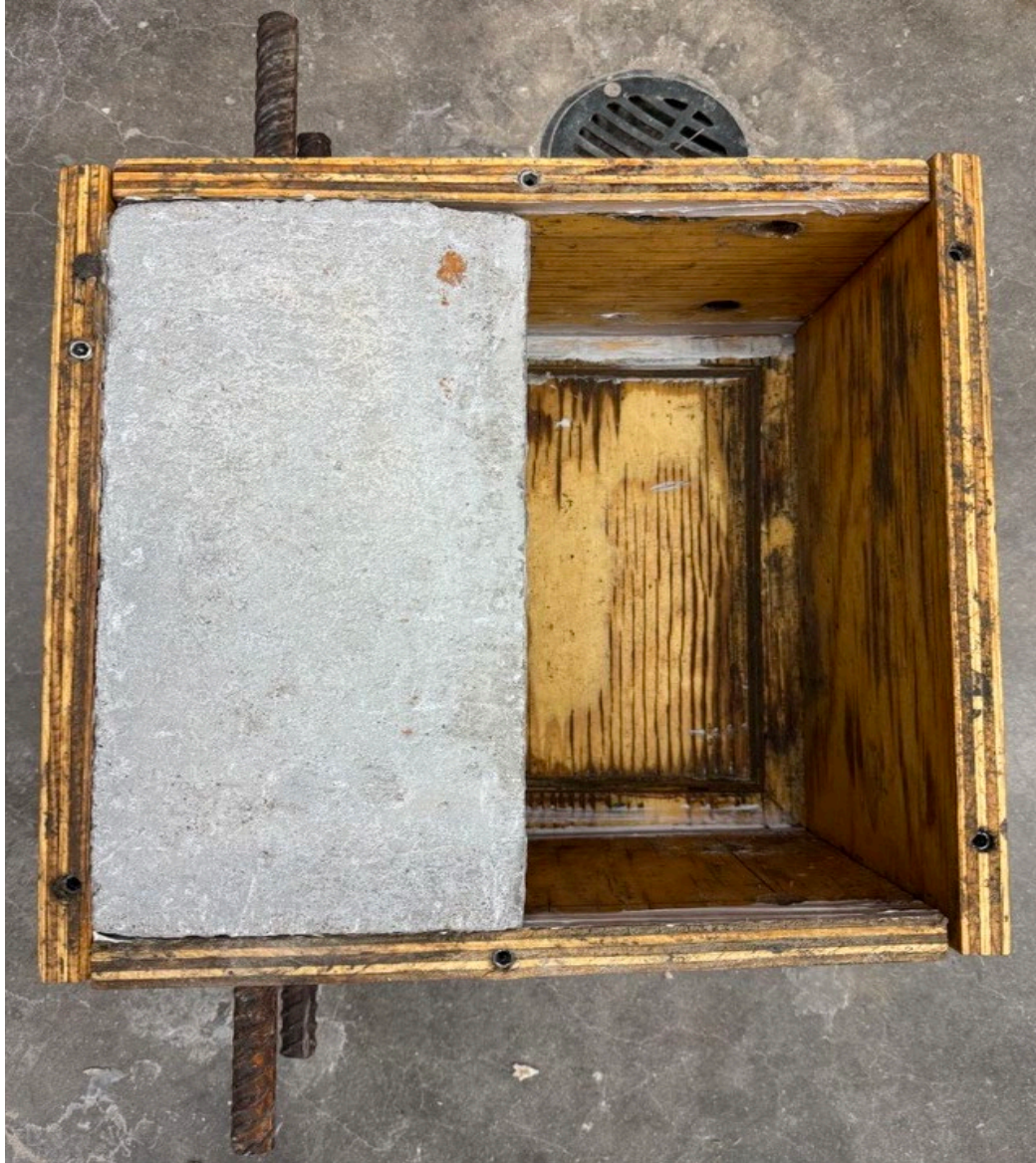
Figure 6: Formwork orientation to cast second half of post-crack specimen
