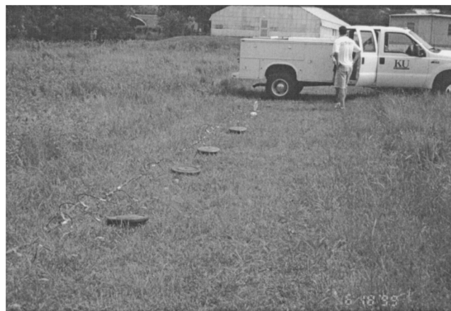
FIG. 1. The various weights balanced on the tops of the 100-Hz vertical geophones include (from front to back) two 22.7-kg and two 11.3-kg circular barbell weights, an 8.2-kg bag of lead shot, a truck, and two 1.1-kg barbell weights (behind the truck).
