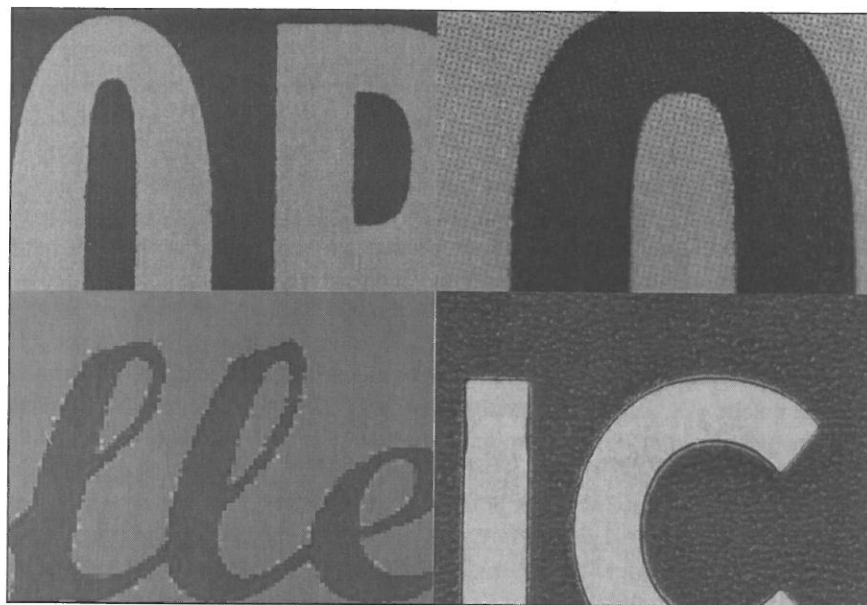
Figure 1. Magnified images of bumper sticker printing processes. Clockwise from top left: screenprinting, offset lithography, flexography, and inkjet. Photograph by the author.
