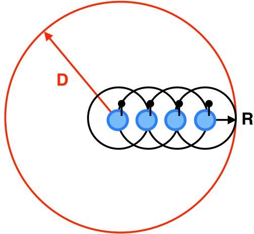
**Figure 5.** The power required to transmit over distance  $D$  increases by a polynomial factor as  $D$  increases. Hopping the data by a distance of  $R$  from pod to pod is more power efficient than directly transmitting the data over distance  $D$ .
