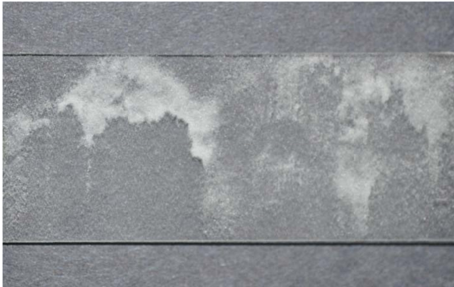
Figure 4.3: Distributed Glass Microspheres on Slide (scale 2:1)
