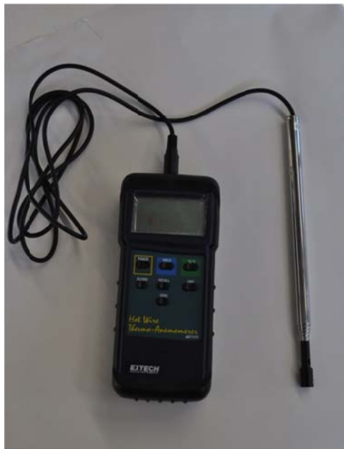
Figure 3.17: Extech 407123 Hot Wire Anemometer
