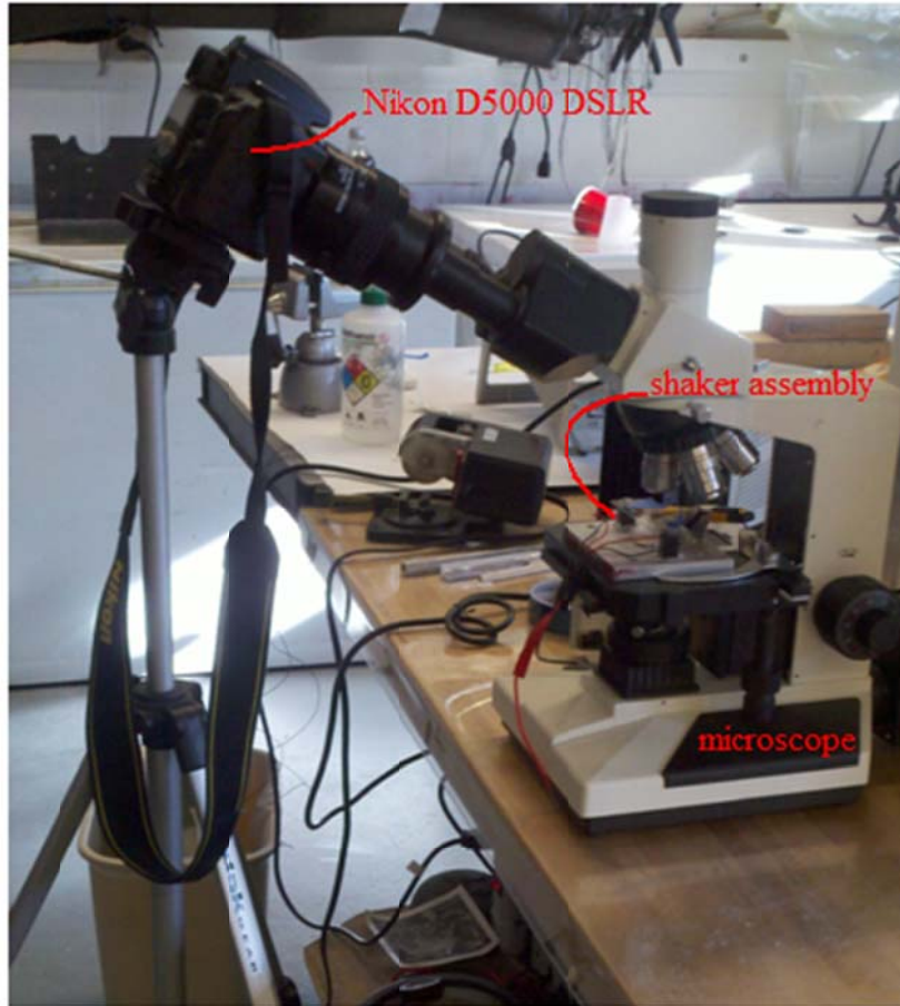
Figure 3.19: Microscope and Camera Positioning
