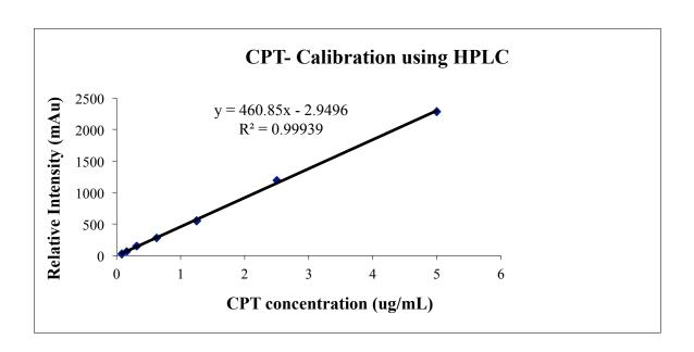
**Figure 3.7.** This calibration plot by HPLC was used to determine drug loading for CPT in the cytotoxicity samples because the drug levels were too low to be detected by UV-Vis spectroscopy.
