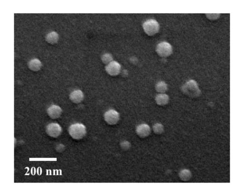
**Figure 2.4.** The SEM image shows particle morphology of hybrid nanoparticles with Egg PC as the lipid.
