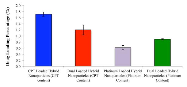
**Figure 3.6.** This graph shows the drug loading results for both camptothecin and Platinum separately as control nanoparticles and dually loaded in combination nanoparticles.
