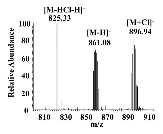
**Figure 3.3.** Electrospray ionization mass spectrometry shows the mass to charge ratios of the Pt-lipid complex.
