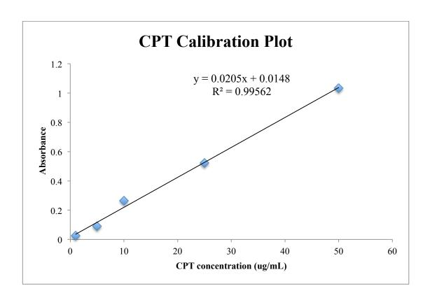
**Figure 3.8.** UV-Vis spectroscopy was used to determine CPT content during the in vitro release studies.
