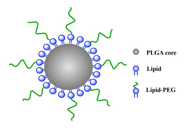
**Figure 1.3.** This diagram shows a representation of the anatomy of a lipid-polymer hybrid nanoparticle.
