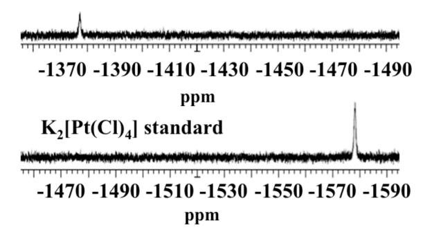
**Figure 3.2.** <sup>195</sup>Pt NMR spectra show the chemical shift for the prepared Pt-lipid compound is different from that of the platinum standard, which indicates that a new chemical entity was synthesized.
