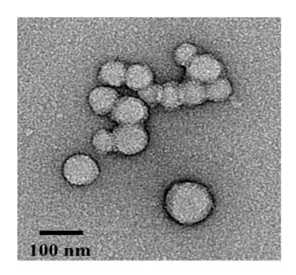
**Figure 2.5.** The TEM micrograph shows the internal structure of the hybrid nanoparticles with Egg PC as the lipid.
