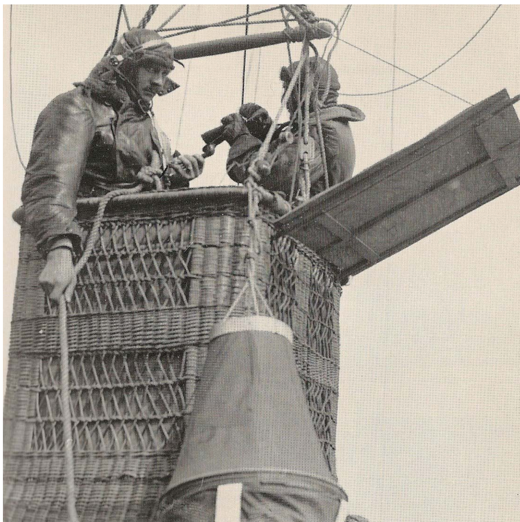
RFC Balloon observer's preparing to ascend. The canvas bag contains the parachute for the observer on the left. http://www.firstworldwar.com/airwar/observation
