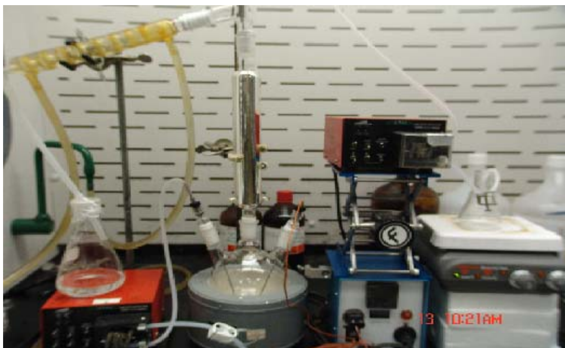
Figure 6.2 Experimental setup of reactive distillation reactor for biodiesel synthesis via transesterification of canola oil with methanol
