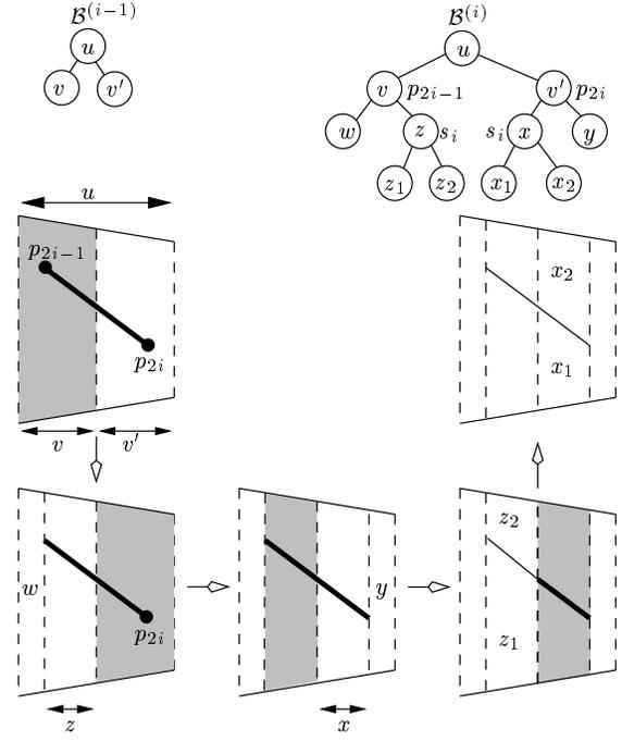
Figure 1: The BSP  $\mathcal{B}^{(i-1)}$ , the sequence of cuts made in the  $i$ th stage, and BSP  $\mathcal{B}^{(i)}$ . At each step, the shaded trapezoids are split. Portions of  $s_i$  that lie in the interior of a trapezoid are drawn using thick lines.
