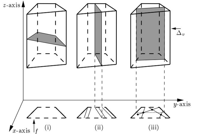
Figure 10: Cuts made in the deterministic algorithm: (i) Free cut, (ii) Cut parallel to the  $z$ -axis through an anchored edge, and (iii) Cut parallel to the  $yz$ -plane through a vertex of  $\mathcal{A}(E_v^*)$
