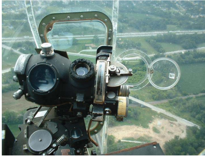
Figure 3. A Norden Mark XV M-1 bombsight in the nose of a B-17G. Source: Author’s collection.
