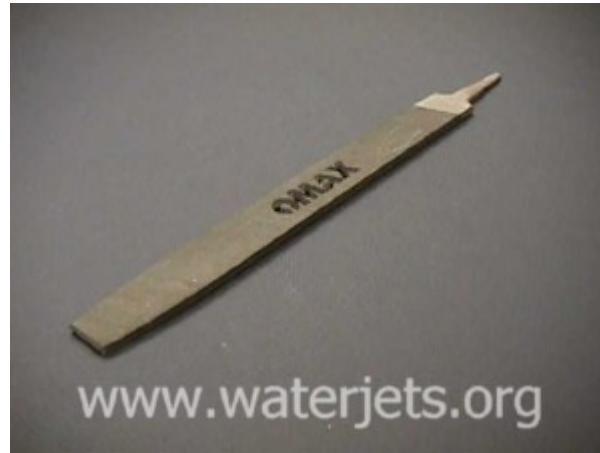
Five minutes is all it took to make this custom file
