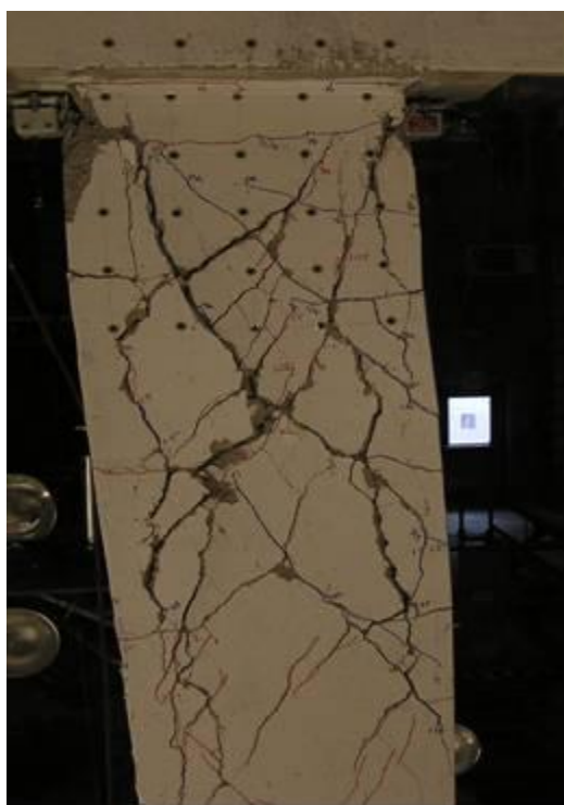
Figure 3.16: Crack pattern at the top of Specimen 4 for a maximum drift ratio of 2%.
