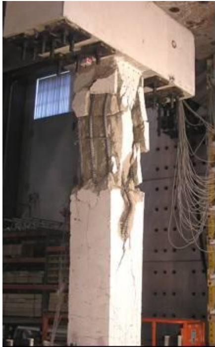
Figure 3.7: Condition of Specimen 3 after a maximum drift ratio of 2%.
