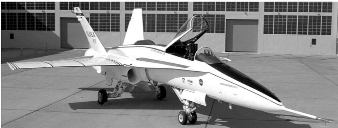
**Figure 2.37 F-18 Employing Active Aeroelastic Wings [86]**
