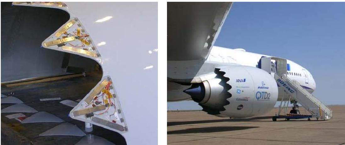
**Figure 2.3 SMA-Actuated Variable Geometry Chevron for Jet Noise Reduction [17]**
