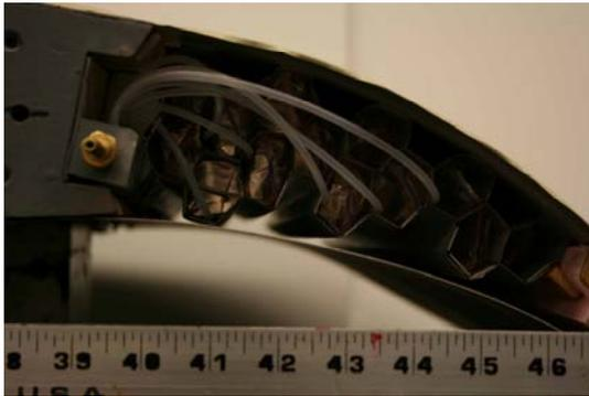
**Figure 5.24 Detail of Pressure adaptive Honeycomb**
