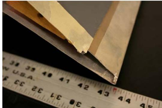
**Figure 5.25 Detail of Sliding Trailing Edge**
