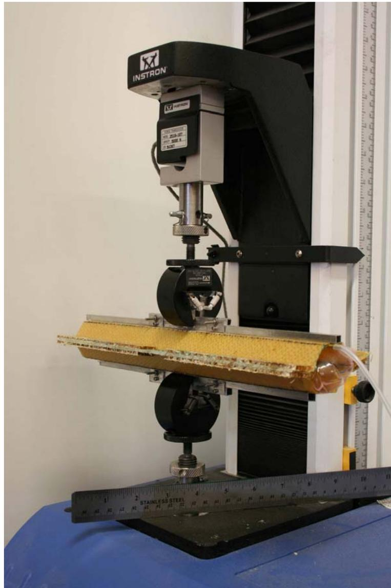
**Figure 5.7** Single Cell Experimental Setup
