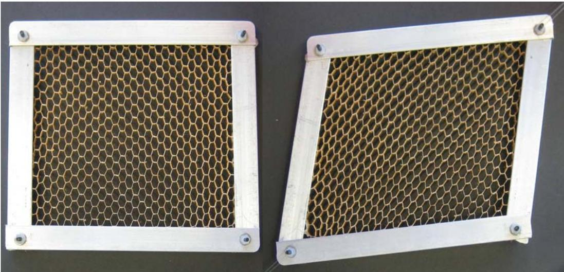
**Figure 4.3 Simple Test Setup To Verify Honeycomb Cell Deformation During Shear Loading**
