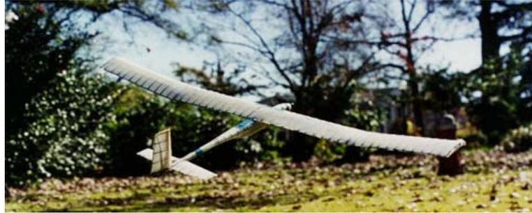
**Figure 2.7** Mothra, the First Aircraft to Fly Using Piezoelectric Flexspar Actuators for All Flight Control [24]
