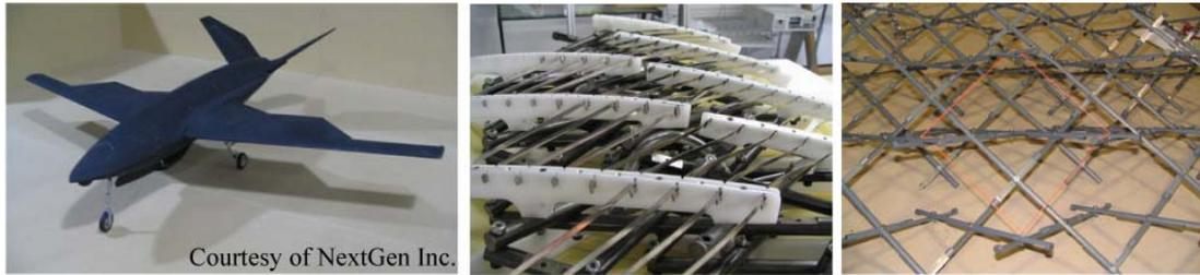
**Figure 2.42 Example of Planform Morphing Wing and Details of Wing Structure [96]**
