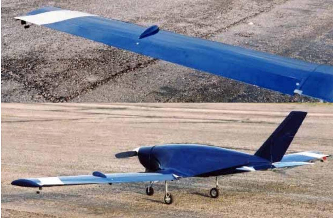
**Figure 2.38** Experimental Aircraft with Operational Twisterons (3.2m span) [93]
