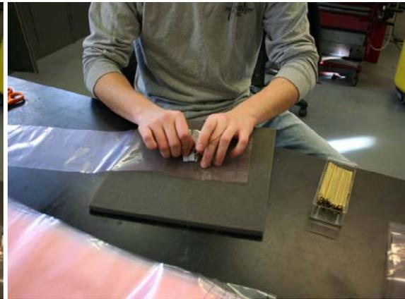
**Figure D. 6** Duct tape patches applied on the outside of the pouch
