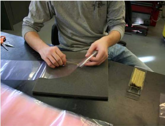
**Figure D. 3** A brass tube is pierced through the plastic
