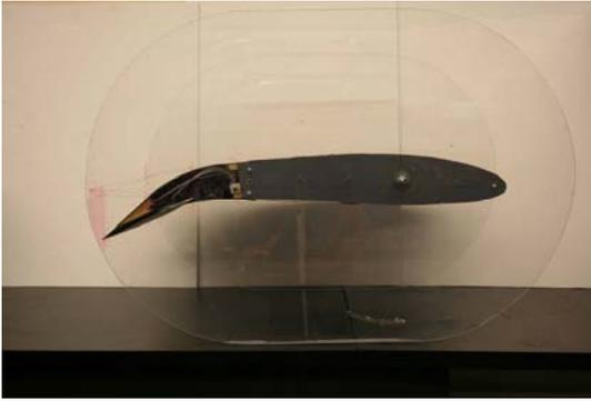
**Figure 5.27** Side View of Model with End Plates
