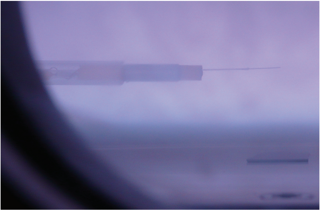
Figure {F-2} Photographs of a probe positioned to measure the presheath (Top, 100% N 2 , 15 mTorr, 50 W) and the bottom of the bulk of the plasma (Bottom, He plasma, 50 mTorr, 100 W) [1].
