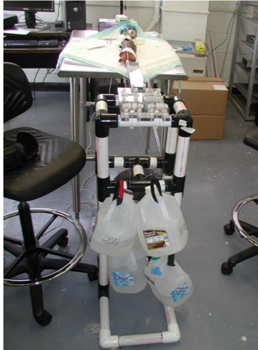
Figure 3.4 Experimental setup showing mechanism for joint loading.
