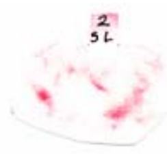
Figure 3.7 Sample template (Specimen 3) showing radioscapoid (left) and radiolunate (right) contact intensity profiles.
