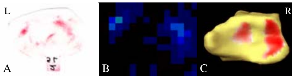
Figure 3.19 Specimen 3 intensity profiles (A) Pressurex, (B) Tekscan and (C) model for lunate (R) and scaphoid (L) contact.
