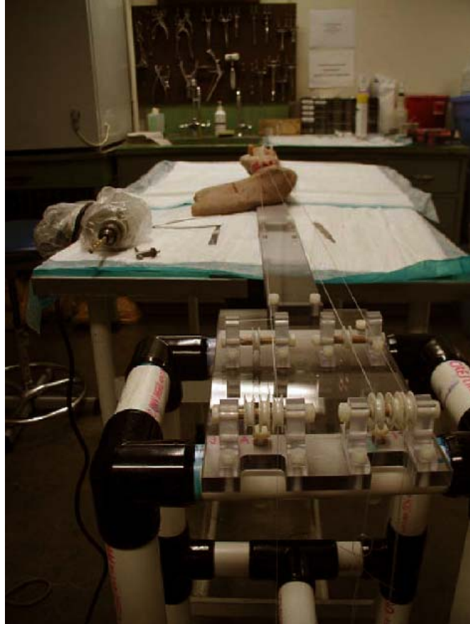
Figure 2.1 Showing mounted specimen and test rig for joint loading.
