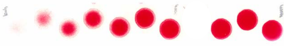
Figure 3.5 Sample calibration data (Specimen 3) from Pressurex sensor.
