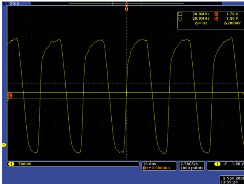
Figure 21: Repeater Input Signal Integrity Results
