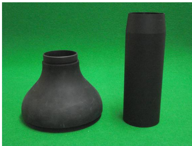
Figure 3.36 Fabricated subsonic nozzle and reducer (outer)
