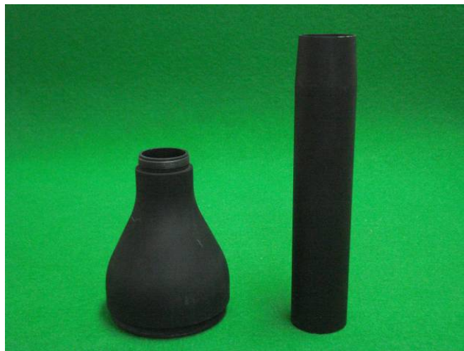
Figure 3.33 Fabricated subsonic nozzle and reducer (inner)
