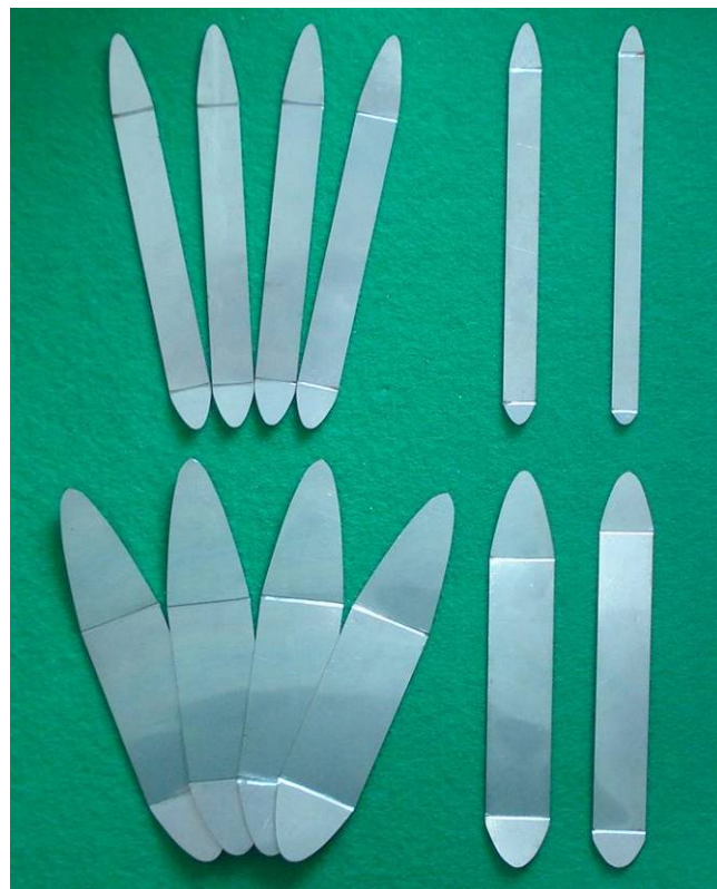
Figure 3.29 Photograph of excitation devices for inner jet (upper) and outer jet (lower)
