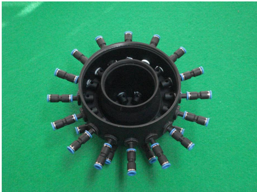
Figure 3.26 Installed swirl injectors (inner and outer) rear view (upper), front view (lower)
