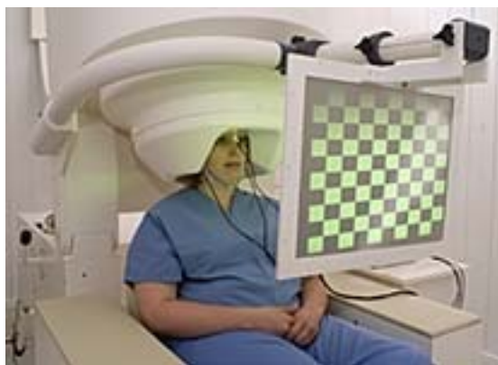
Figure 2-3. Biomagnetometer system with 151 channels during cortical MEG recording at the Hoglund Brain Imaging Center in KUMC
