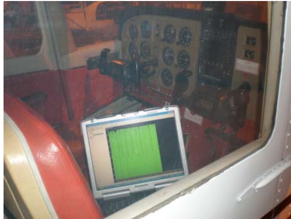
Figure 5-13: CDU Placed inside C-172 for Signal Strength Measurement
