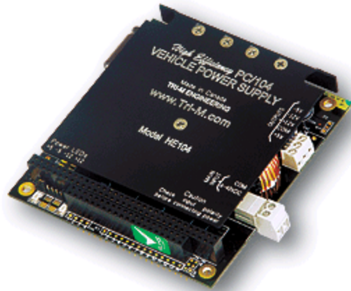
Figure 3-5: HE104-512-16 PC/104 Power Supply
