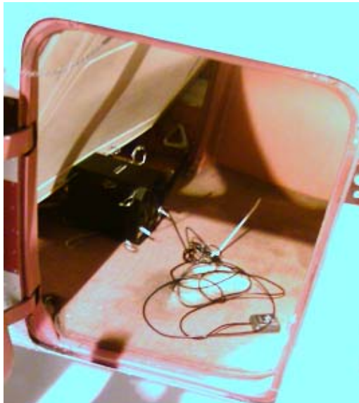
Figure 5-19: Wireless AHRS Unit Installed in the Luggage Compartment of C-172
