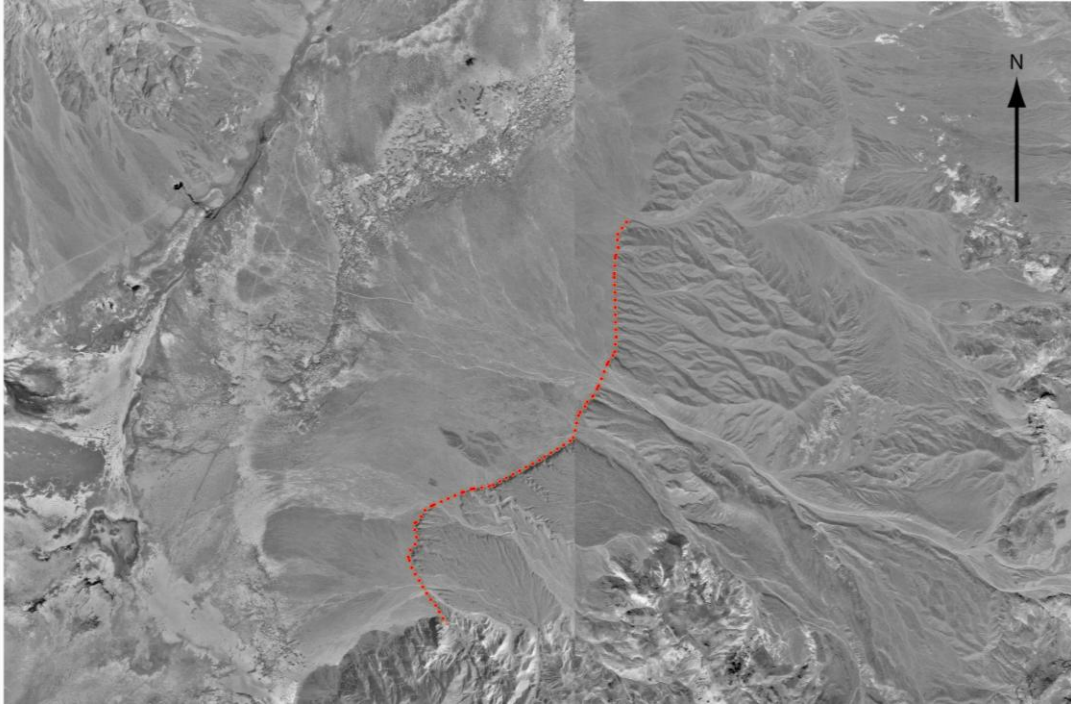
Figure 1. Aerial photograph of the EMPZ. The red, dashed line represents the location of the present fault scarp.
