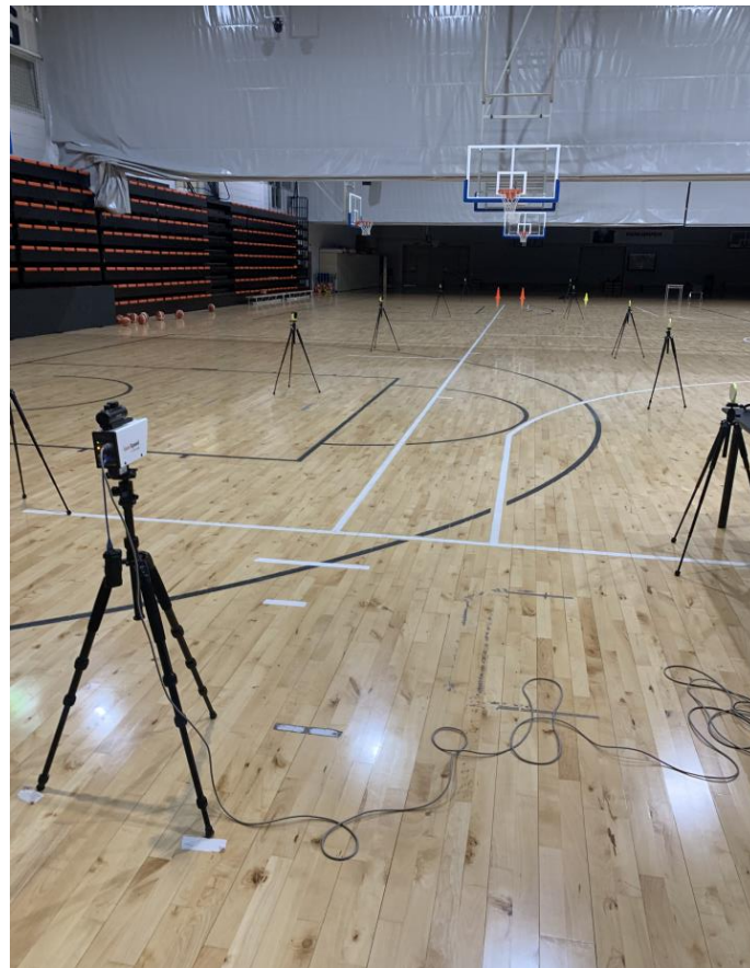
Figure 9. Laser gun and timing gates setup.
