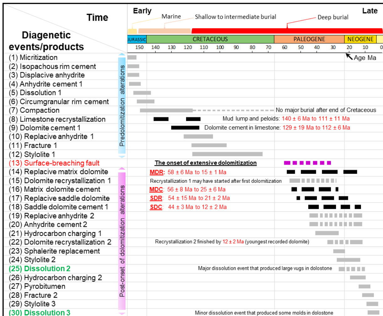
Figure 4.11. Paragenesis of the Upper Jurassic Arab Formation in northeast Saudi Arabia. The diagenetic history of the carbonates can be grouped generally into predolomitization and post onset of dolomitization stages. Bars in black are constrained by U–Pb dating with the ages provided by the red text. All other events are constrained by cross-cutting relationships, geochemical analyses, and knowledge of published structural and burial history of the region.
