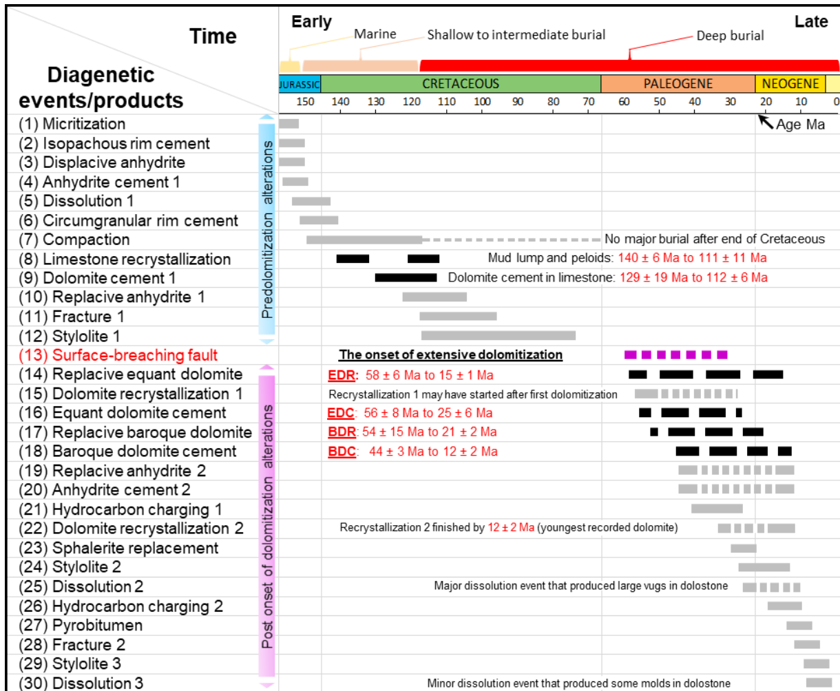
Figure 2.15. Paragenesis of the Upper Jurassic Arab Formation in northeast Saudi Arabia. The diagenetic history of the carbonates can be grouped generally into predolomitization and post onset of dolomitization events. The extensive dolomitization that produced the bulk of dolomite is the main diagenetic event. Bars in black are constrained by U–Pb dating with the ages provided by the red text. All other events are constrained by cross-cutting relationships, geochemical analyses, and knowledge of published structural and burial history of the region.
