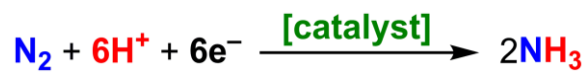
Figure 2.23: Reduction of dinitrogen using protons and electrons in combination with an electrocatalyst to generate ammonia.
