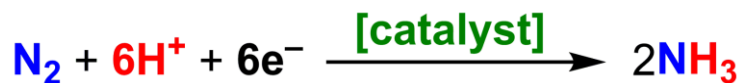
Figure 2.23: Reduction of dinitrogen using protons and electrons in combination with an electrocatalyst to generate ammonia.
