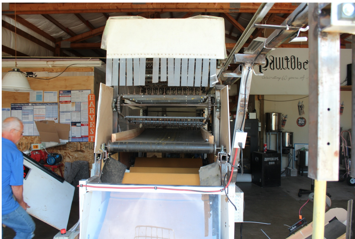
Figure 4-1: Homemade Hop Picker, Patrick removes plywood cover to show interior picking teeth and belt mechanisms. Manufactured hop pickers for 10 acres or less often cost ~$10000 and up. Patrick Reports building this picker for less than $1500.
