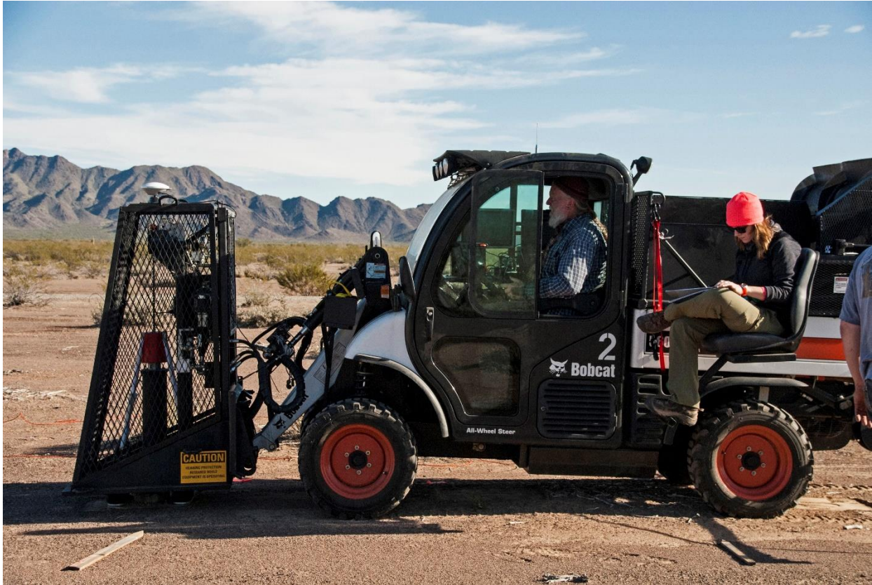
Figure 7. Photograph of the accelerated weight drop source mounted to the front of a modified Bobcat. Photo courtesy of Kansas Geological Survey.
