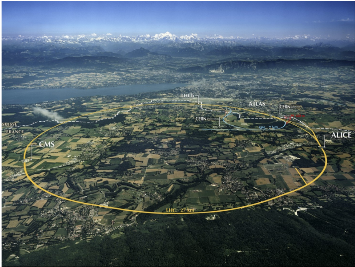
Figure 2.1: A satellite photo of the LHC complex at surface level. Each of the 4 main experiments is shown. The actual ring itself is located underground at depths of up to 175 meters.
