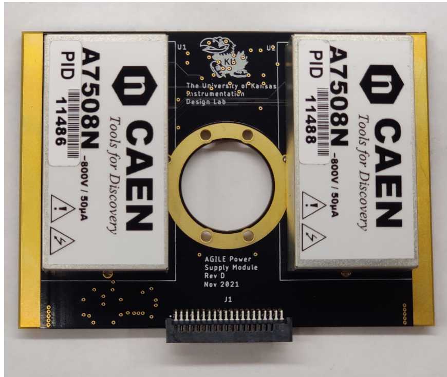
Figure 4.25: Power supply board for AGILE detectors bias voltage distribution. The board hosts one main and one redundant CAEN A7508 units. The input 5 V are converted to around 100 V output to the silicon sensors hosted in the three detection layers.
