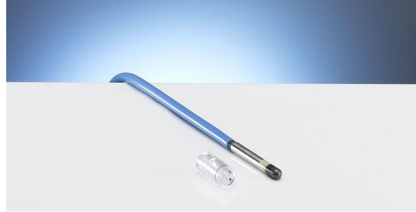
Figure 3.11: Picture of the PTW Semiflex ionization chamber 31010 encapsulated in the PMMA cylinder.
