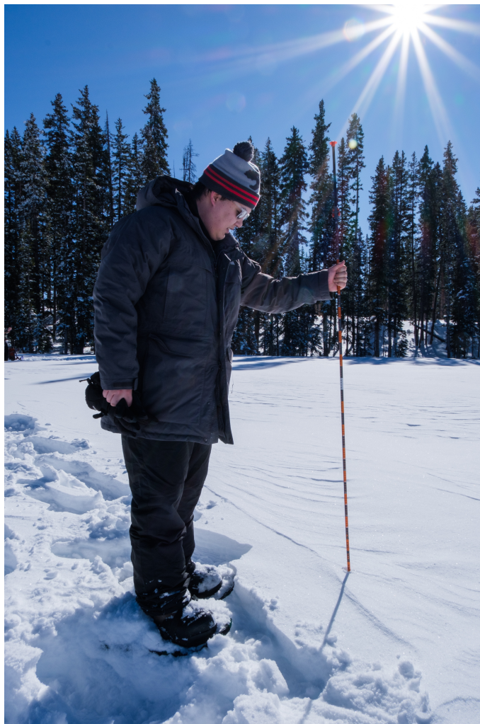
Figure 2.1: Image of depth measurement from Jan 2020 field survey of snowpack in Grand Mesa, Colorado using a 3 m avalanche pole.
