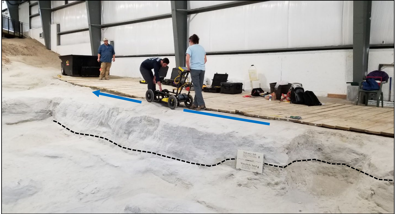
Figure 3. 1: Image of the 500 MHz frequency antenna deployed to test the depth to sandstone along the known sandstone contact (dashed line).
