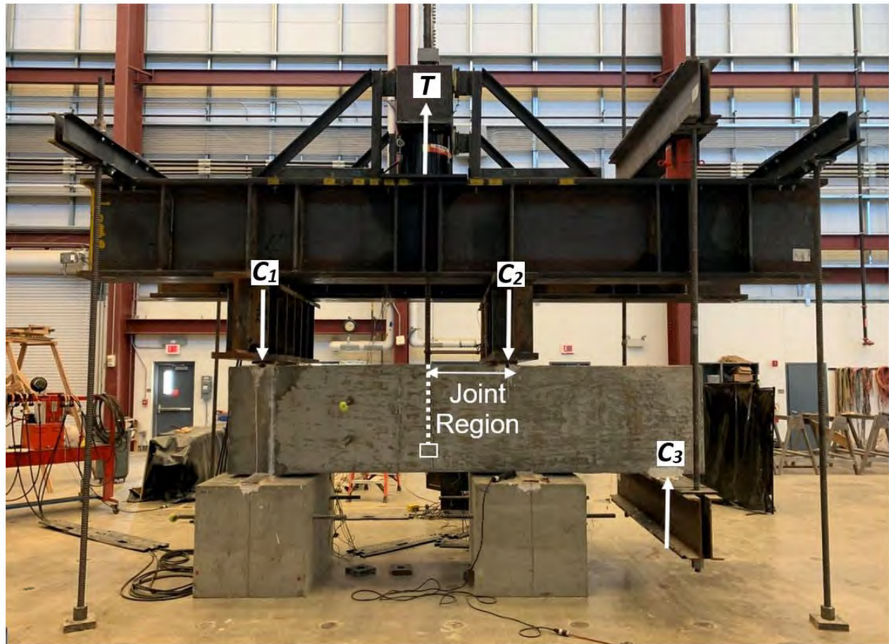
Figure 2.18 The reaction frame (No. 14 bar setup) and applied forces
