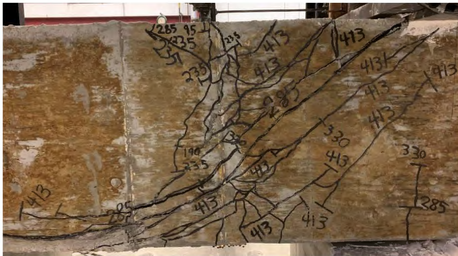
Figure 5.29 Concrete breakout observed in specimen 14-17 ( A_{tr}/A_{hs} = 0.551 ) with increased side cover to the bar and decreased bar spacing
