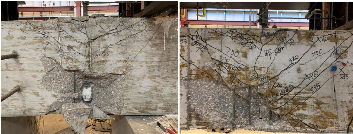
Figure 3.8 Primarily side-splitting failure (left: specimen 14-3, right: specimen 18-4)
