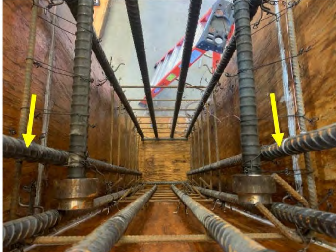
Figure 5.16 Additional No. 11 longitudinal bars in specimen 14-16A
