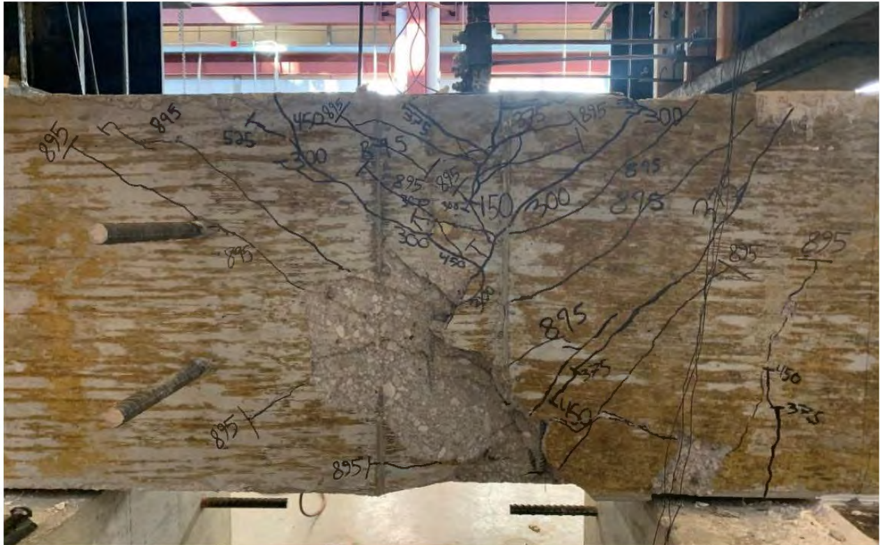
Figure 3.6 Side view of a side-splitting failure for hooked bars (H14-8)
