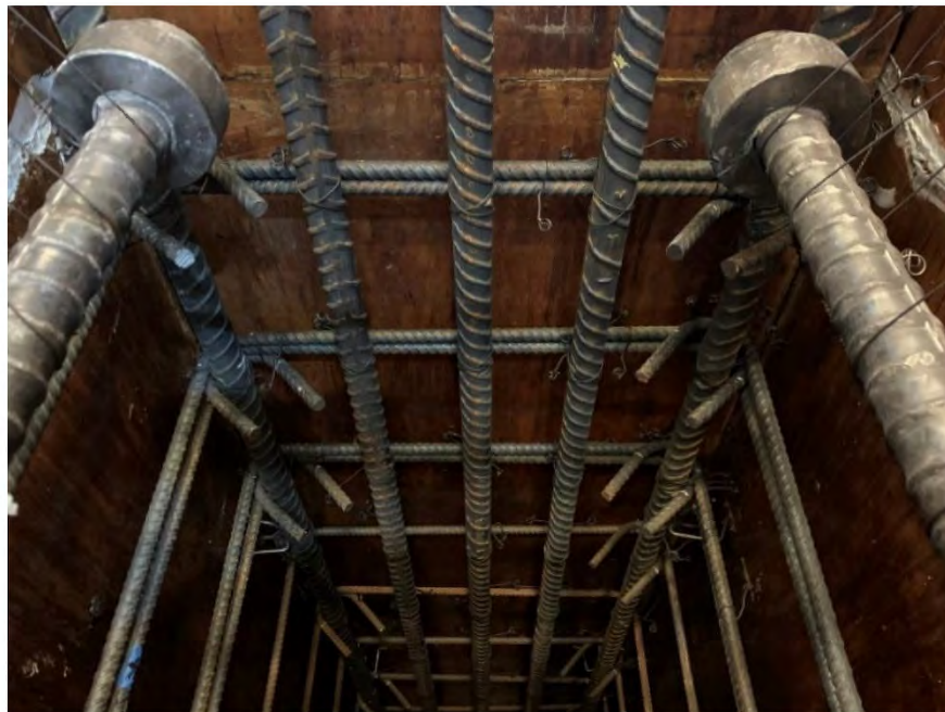
Figure 5.26 Double No. 5 ties used in specimen 14-16F
