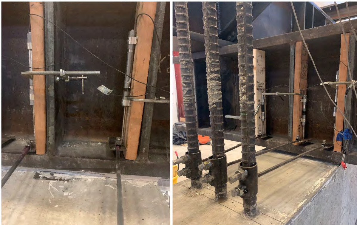
Figure 2.22 Setup for using the LVDTs
