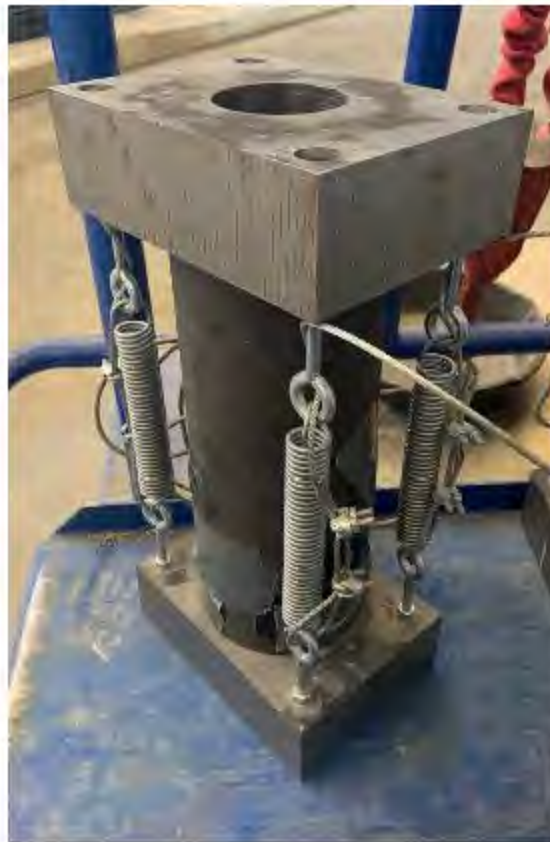
Figure 2.23 Load cell for No. 14 and No. 18 bars
