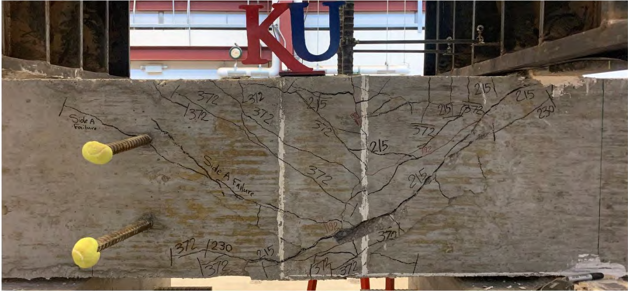
Figure 3.9 Combination of concrete breakout and side splitting (specimen 14-15)
