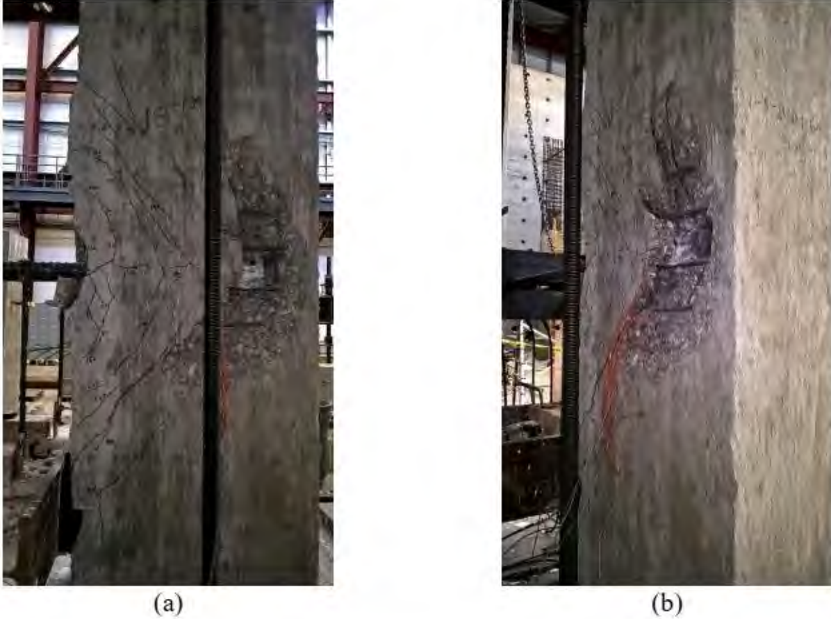
Figure 1.18 Side-face blowout (a) side view (b) back view (Shao et al. 2016)
