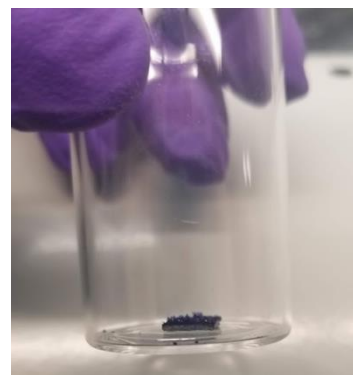
Figure 4.10: An overdosed azulene on graphite sample. A dark blue layer of azulene, with some large crystals, is visible on graphite's dark grey surface.
