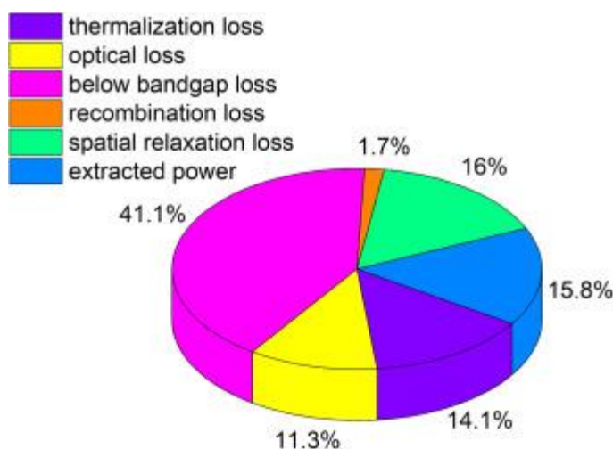
Figure 9: Quantification of energy loss occurring in the perovskite solar cells under AM1.5 illumination. 30 . Reprinted from Solar Energy Materials and Solar Cells , Vol 174, Yun Da, Yimin Xuan, Qiang Li, Quantifying energy losses in planar perovskite solar cell, 206-213, Copyright (2023), with permission from Elsevier.
