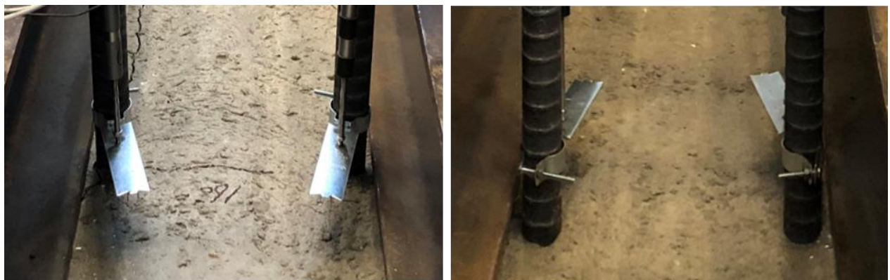
Figure 2.16 LVDT plates attached to test bars
