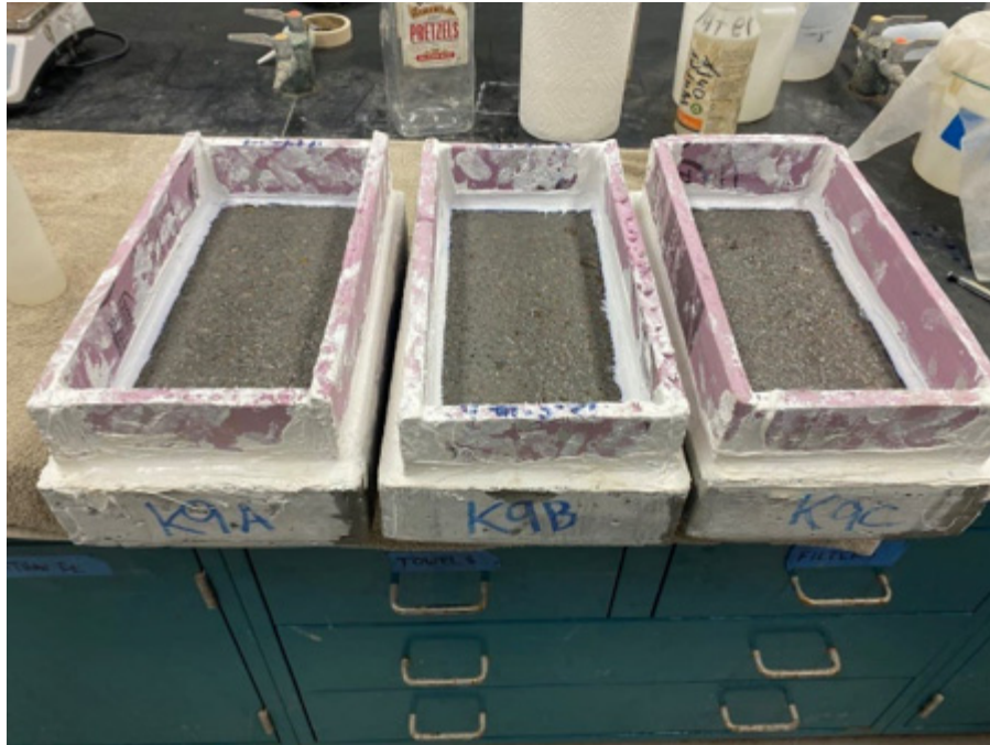
Figure 2.5: Scaling specimens with polystyrene foam dikes attached
