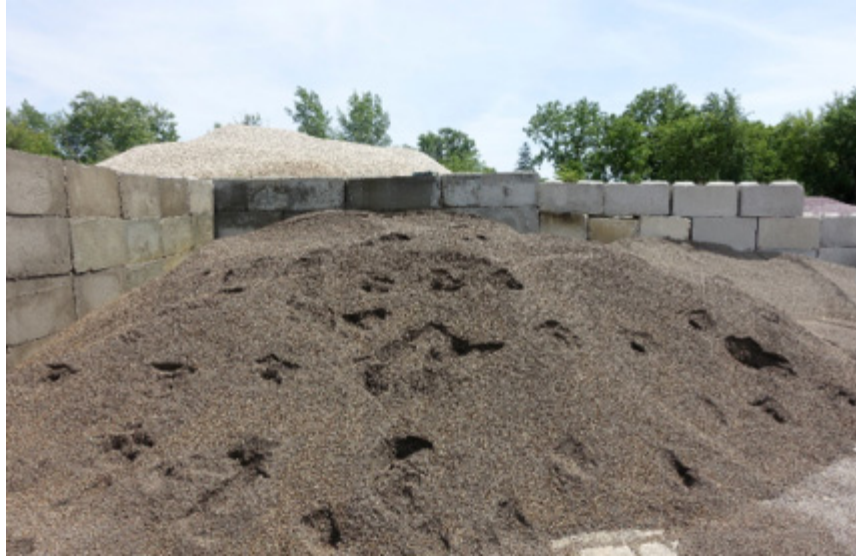
Figure 4.1: Lightweight aggregate stockpile for MN-IC-LC-HPC-2
