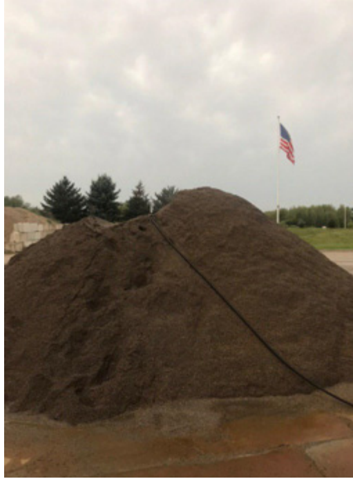
Figure 4.15: Lightweight aggregate stockpile for MN-IC-LC-HPC-6
