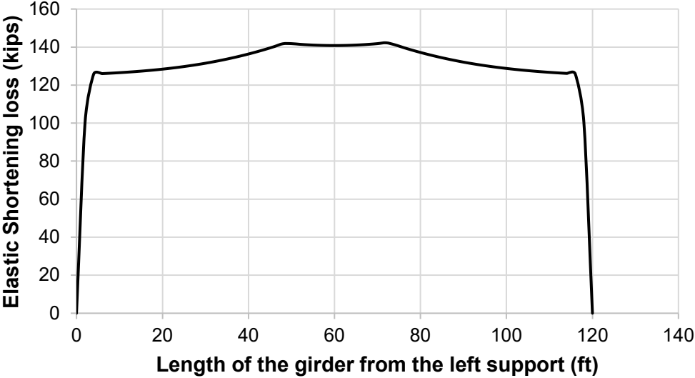
Figure 4.6: Elastic-Shortening Loss Throughout the Girder Length
