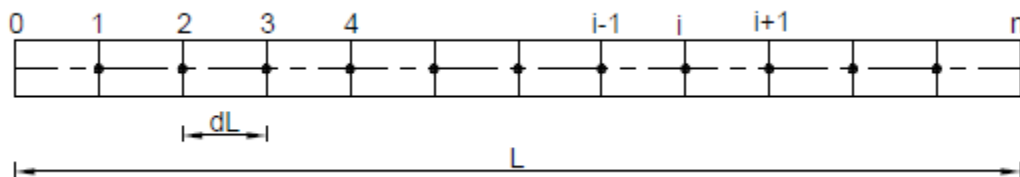
Figure 3.10: Division of Girder into Segments for Analysis
