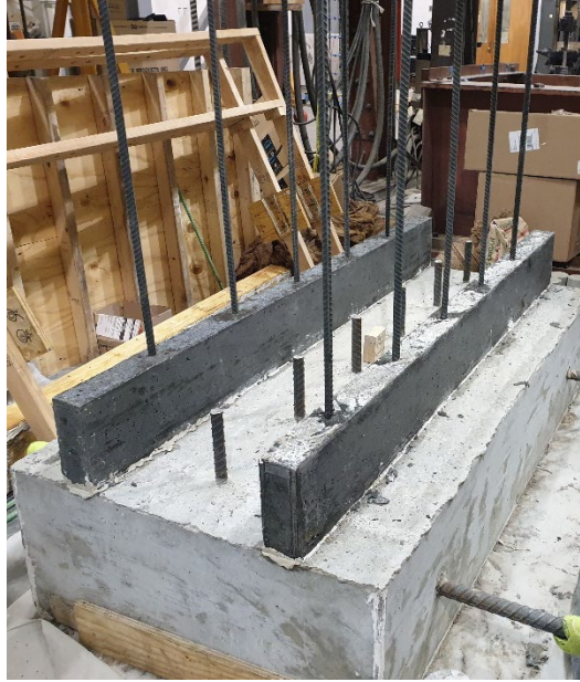
Figure 2.11: Pullout Specimens cast on Base Slab 4
