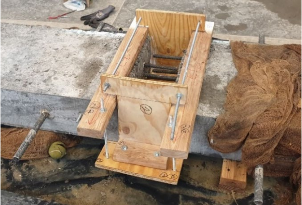
Figure 2.21: Formwork for Casting UHPC Strip for Beam-Splice Specimen
