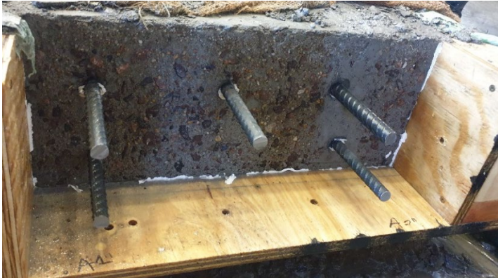
Figure 2.20: Exposed Aggregate Look of Side Panel
