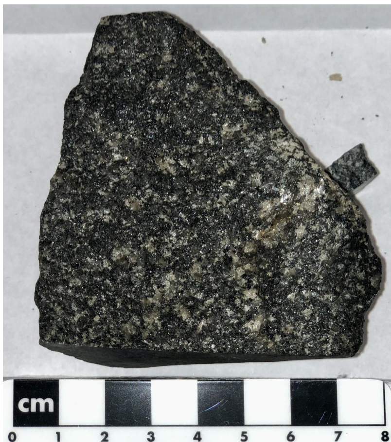
Figure 6: Photograph of the MC-5 hand sample. Note the distinct resinous luster due to high garnet content. The dark color made it difficult to identify specific minerals in hand sample. The rock weathers to a mottled gray and black.
