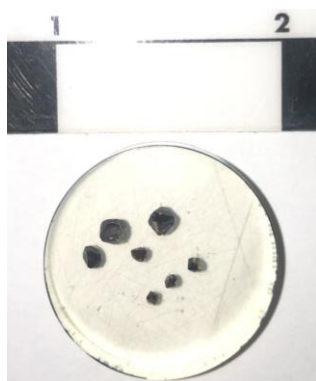
Figure 4: Magnet Cove perovskite mounted in 1-inch round of clear epoxy for analysis by LA-ICP-MS.
