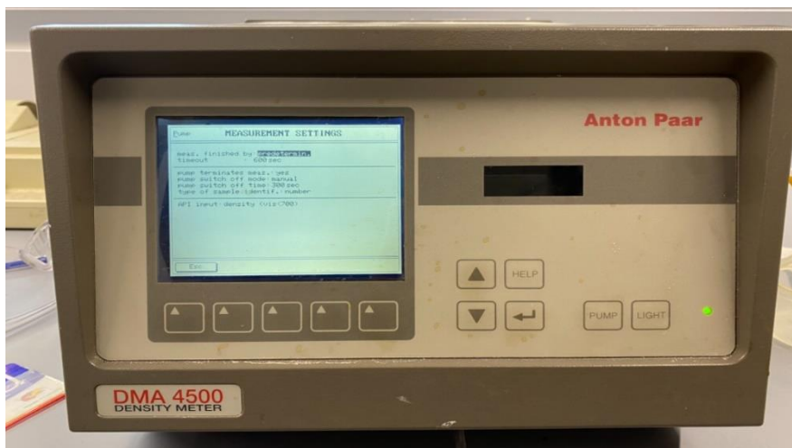
Figure 8. Densimeter DMA 4500, Anton Paar
