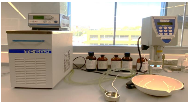
Figure 12. Viscosimeter DV-II + Pro, Brookfield with Thermo-cooling Bath TC-602
