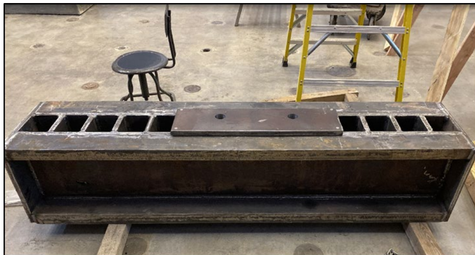
Figure 30 - Washer plate attached to the built-up section
