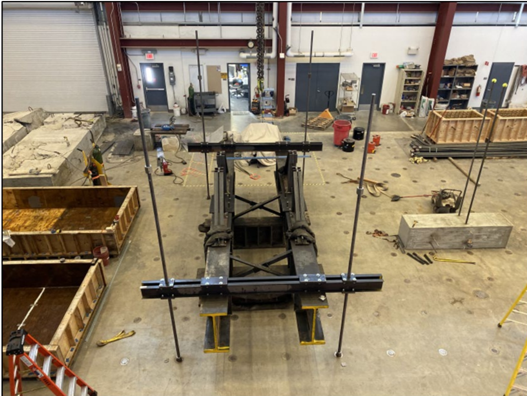
Figure 27 - Reaction frame staging area
