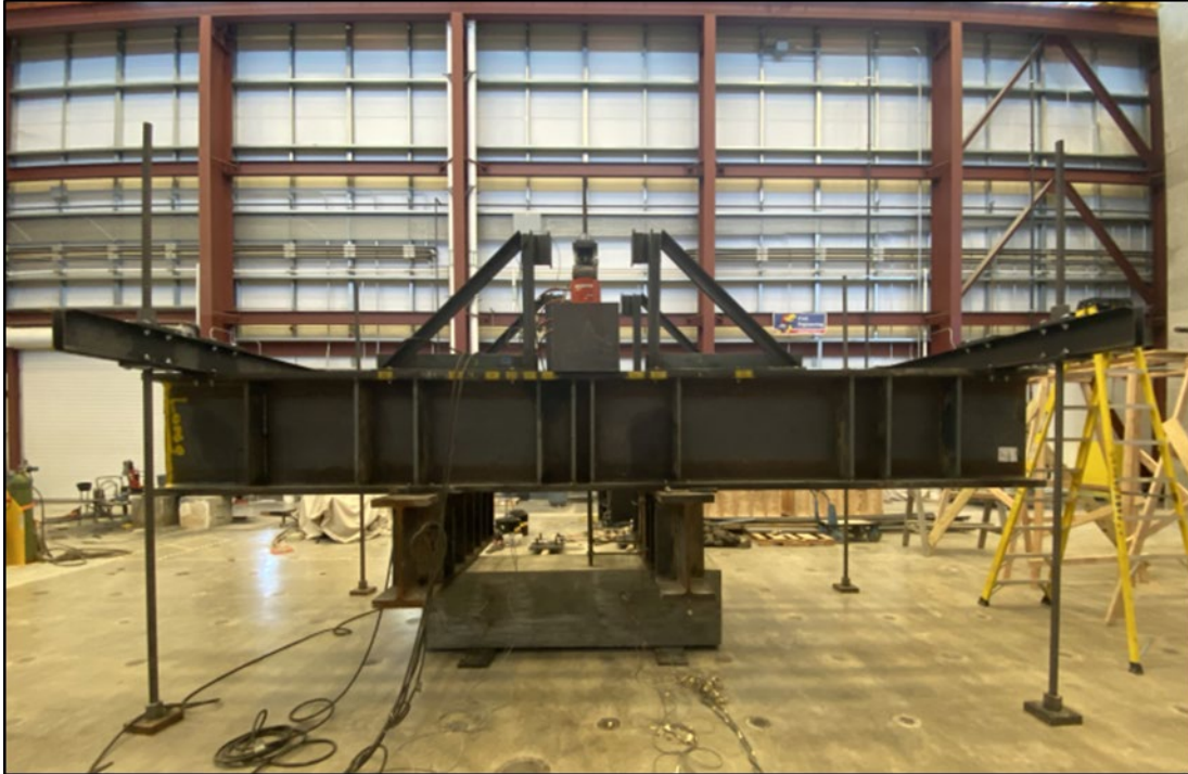
Figure 33 - Reaction frame completed set up side view
