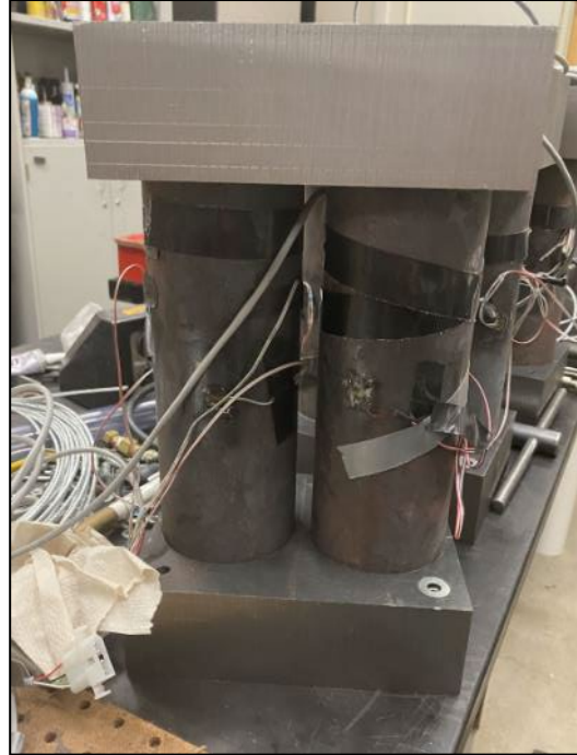
Figure 25 - No. 14 and No. 18 bar two-row load cell
