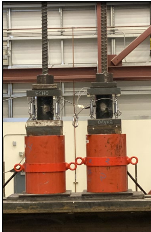
Figure 31 - Hydraulic jack, load cells, and grips on the test bars
