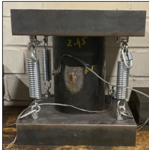
Figure 26 - Initial No. 11 bar load cell
