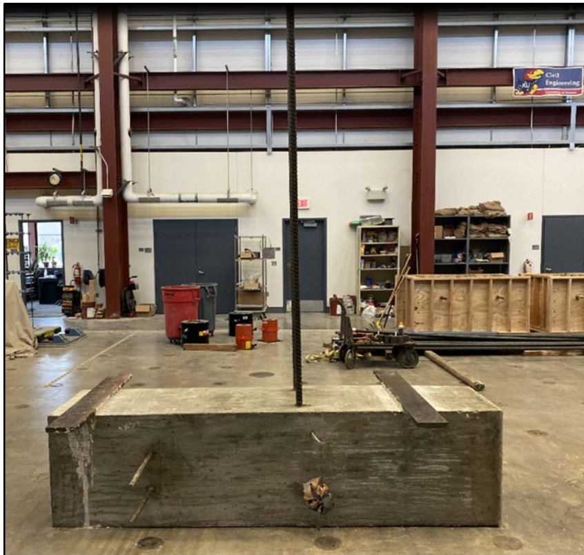
Figure 28 - Bearing plates placed on the specimen with hydrostone
