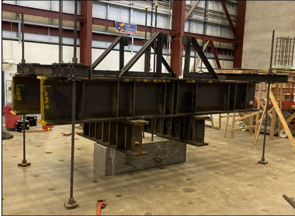
Figure 29 - Reaction frame lifted onto the specimen
