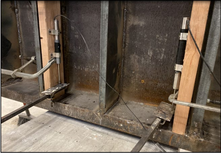
Figure 22 - LVDT clamped to the lower bearing member
