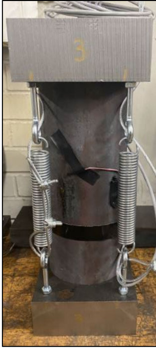
Figure 24 - No. 14 and No. 18 bar single-row load cell
