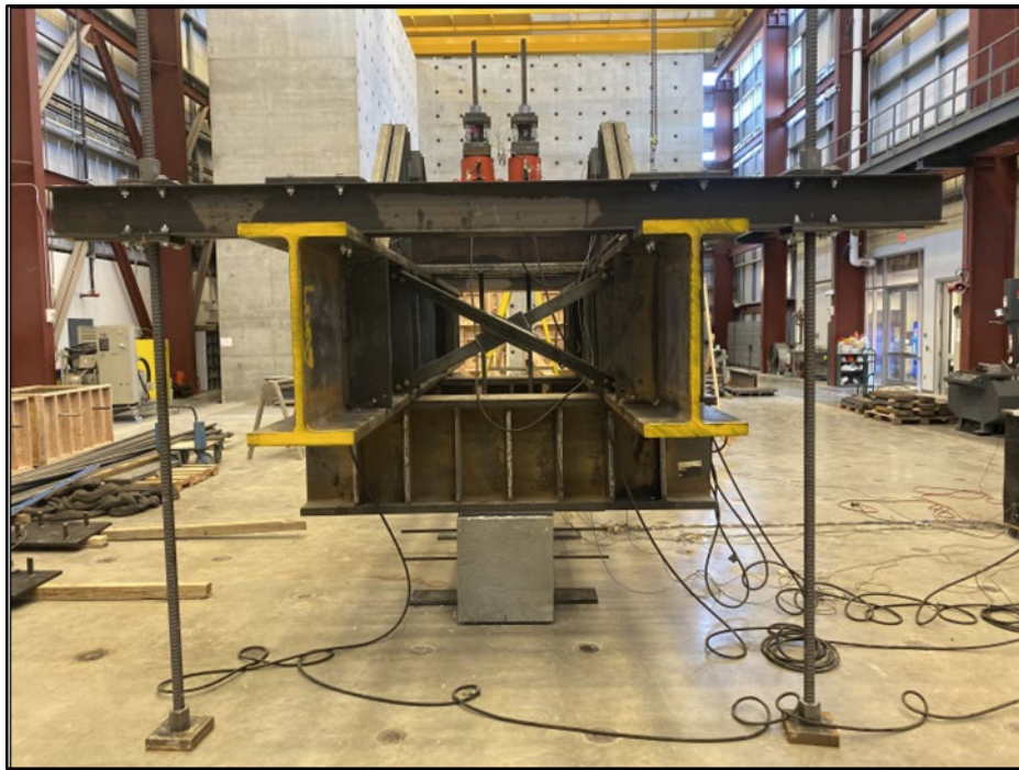
Figure 32 - Reaction frame completed set up top view
