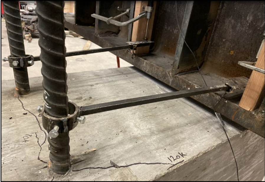
Figure 23 - LVDT HSS attachment to the test bar
