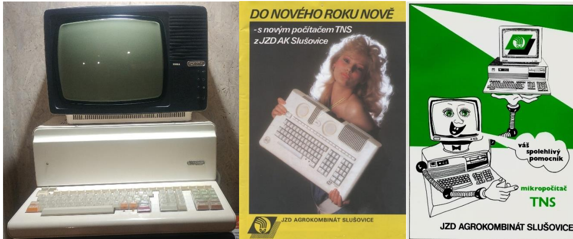
Figure 8: The TNS (Ten Náš Systém) SL-64 workstation, designed and produced in 1986 at the JZD Agrokombinát Slušovice in Moravia. Equipped with a built-in mechanical 5.25" disk drive and typically hooked up to a Tesla Merkur television display as shown here, the agricultural cooperative near Zlín produced and sold several hundred units of this computer inside Czechoslovakia in the late 1980s. Advertisements are a large-scale placard (undated) and full-page print ad from the March 1988 issue of Mikrobáze .
