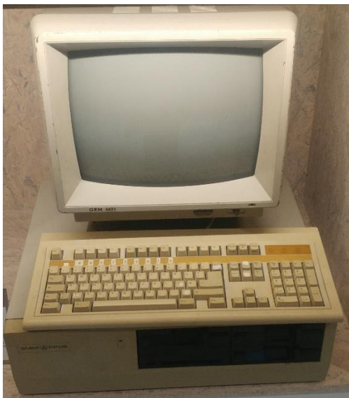
Figure 8: The TNS (Ten Náš Systém) SL-64 workstation, designed and produced in 1986 at the JZD Agrokombinát Slušovice in Moravia. Equipped with a built-in mechanical 5.25" disk drive and typically hooked up to a Tesla Merkur television display as shown here, the agricultural cooperative near Zlín produced and sold several hundred units of this computer inside Czechoslovakia in the late 1980s. Advertisements are a large-scale placard (undated) and full-page print ad from the March 1988 issue of Mikrobáze .
