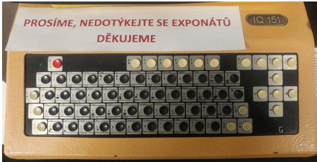
Figure 5: The IQ 151 was inspired by one of the first commercially successful home computers, the Apple II (1977). Production began at ZPA Nový Bor in 1985, intended to supply Czech schools and using the reverse-engineered Tesla MHB8080A microprocessor. However, the IQ 151 was plagued with quality problems, including overheating, a notoriously difficult-to-use keyboard and components so badly fitted to the motherboard that integrated circuits would regularly detach during normal percussive use, i.e. typing.
