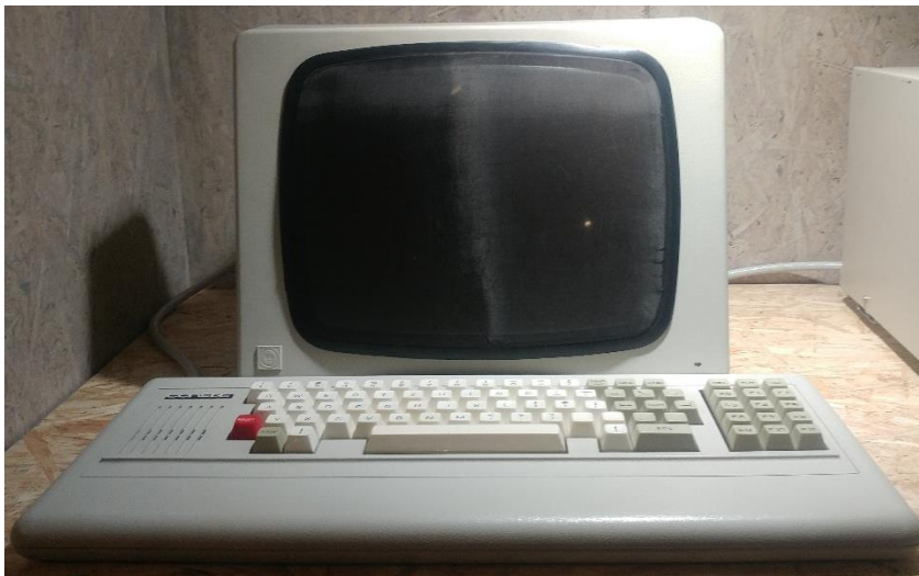
Figure 6: The Consul 2715, produced by Zbrojovka Brno arsenal and office equipment combine in 1983, was a data entry workstation compatible with the IBM 5280 (from 1980). Its CPU was the Tesla MHB 3000, a reverse-engineered clone of the Intel 3000 line of microprocessors from 1974. System RAM varied from 128-512 kB, while initial ROM was limited to 64 kB.
