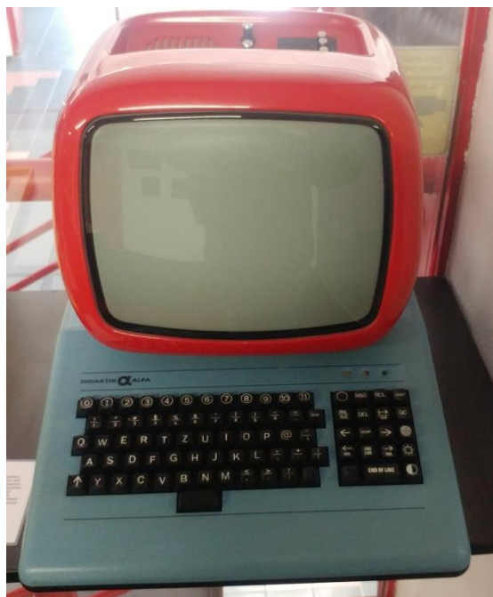
Figure 1: The Didaktik Alfa, a clone of the PMD 85-1 produced in Skalica, Slovakia in 1986 and intended for schools. It used Tesla's reverse-engineered MHB8080A microprocessor and had 48 kB of RAM and 4 kB of ROM.
