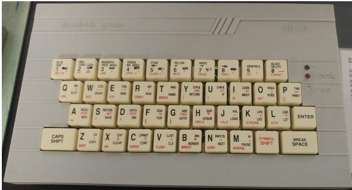
Figure 3: The Didaktik Gama, a clone of the Sinclair ZX Spectrum and the most commercially successful Czechoslovak computer. Mass production began in Skalica, Slovakia in 1987 and continued until 1992. Unlike other Czechoslovak clone computers, the Didaktik ran on an authentic imported Zilog Z80 microprocessor (not the Tesla MHB8080A), 80 kB of RAM and 16 kB of ROM, and thus featured full software compatibility with the extensive library of the British ZX Spectrum.
