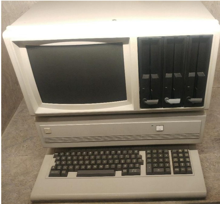
Figure 6: The Consul 2715, produced by Zbrojovka Brno arsenal and office equipment combine in 1983, was a data entry workstation compatible with the IBM 5280 (from 1980). Its CPU was the Tesla MHB 3000, a reverse-engineered clone of the Intel 3000 line of microprocessors from 1974. System RAM varied from 128-512 kB, while initial ROM was limited to 64 kB.
