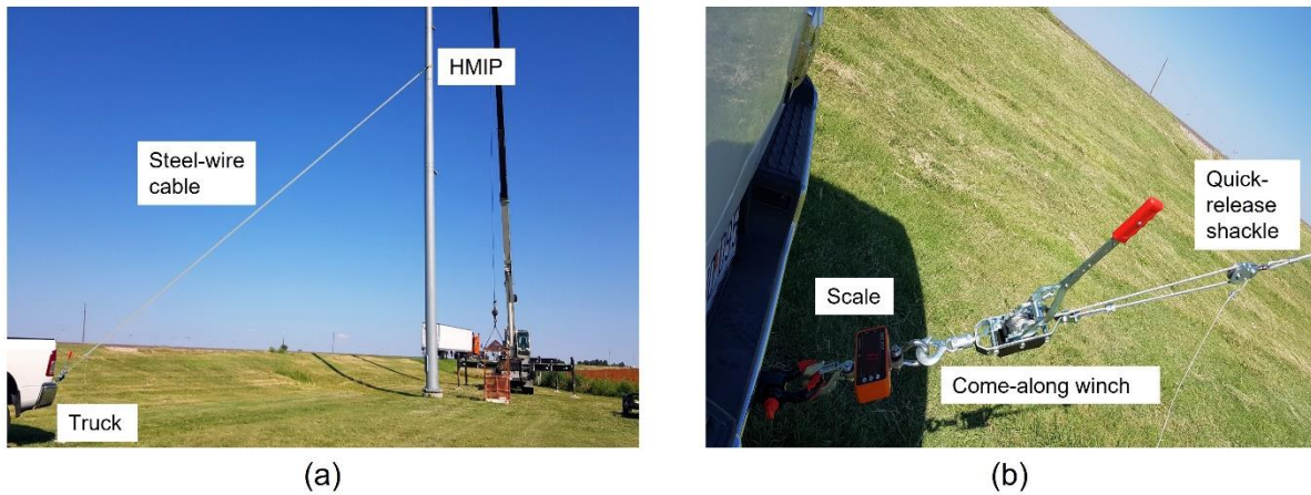
Figure 2-12 (a) Illustration of the pluck tests; (b) Tools used in the pluck tests
