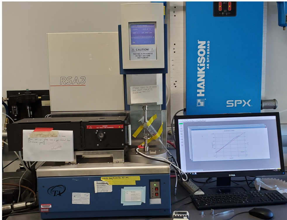
Figure 2.15: TA dynamic mechanical analyzer (RSA III) utilized in the mechanical characterization of the polysaccharide thermoplastic films in Chapter 6.
