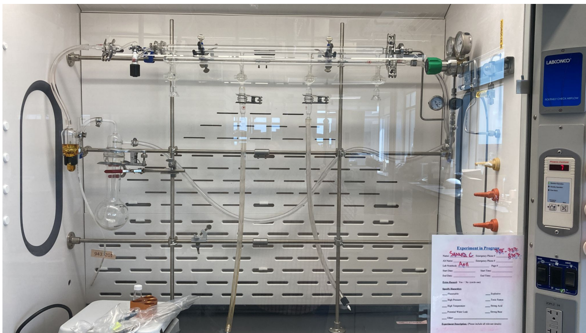
Figure 2.1: A depiction of the Ace Glass Schlenk line used for the synthesis of organometallic complexes used in this body of work.
