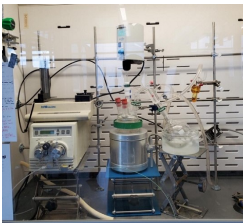
Figure 2.9: 1L kettle reactor with a 5-neck cap utilized in the production of modified \alpha -1,3-glucan materials.
