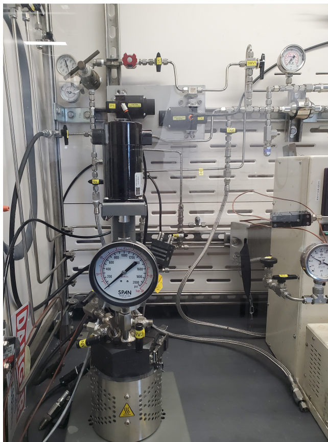
Figure 2.3: 5500 high-pressure compact Parr reactor with a 50 mL cup.
