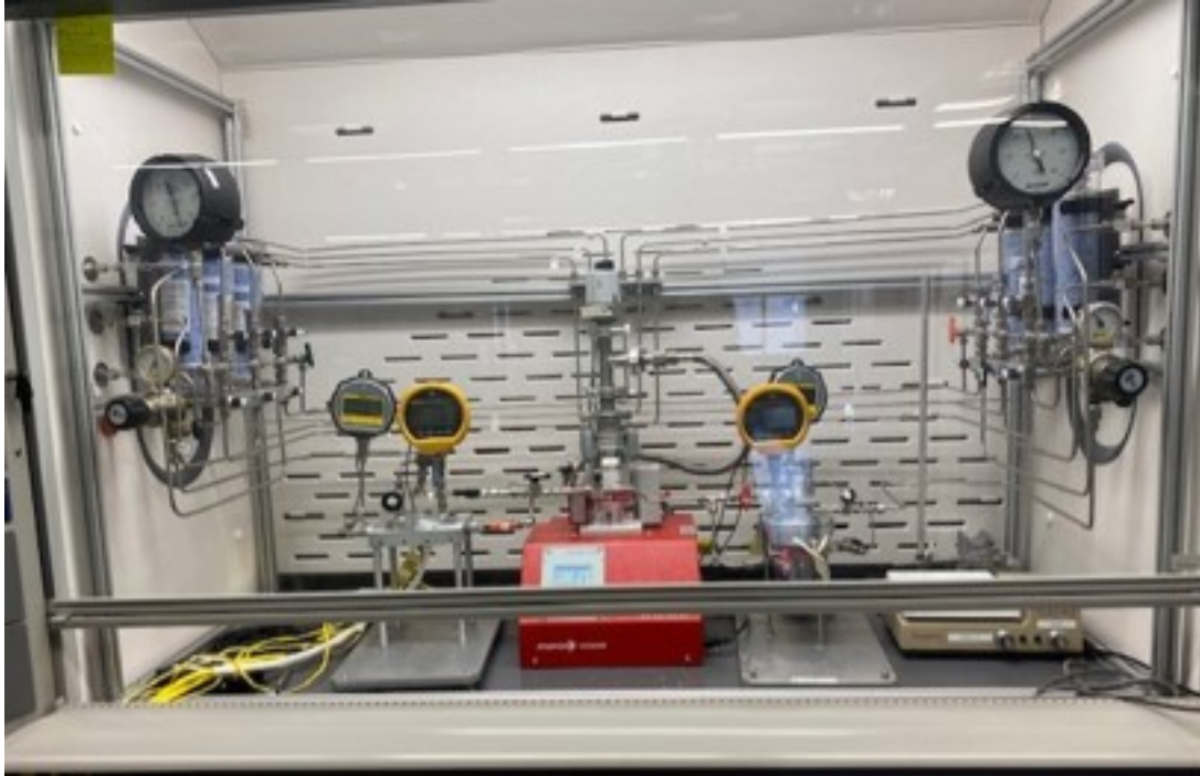
Figure 2.16: Experimental apparatus utilized in the study of gas permeability for a variety of polymeric films.
