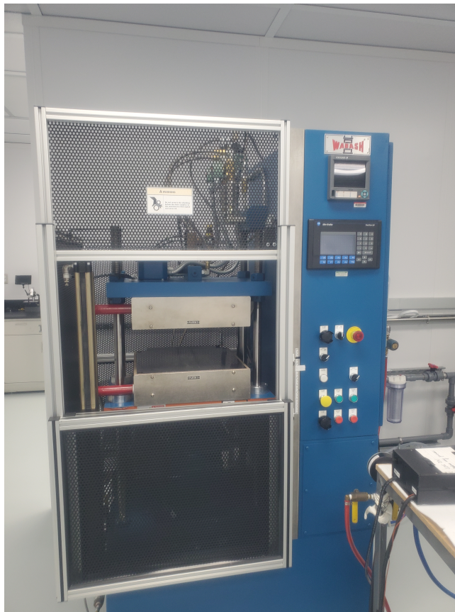
Figure 2.13: Hot press equipment utilized in the fabrication of polysaccharide thermoplastic films in Chapter 6.
