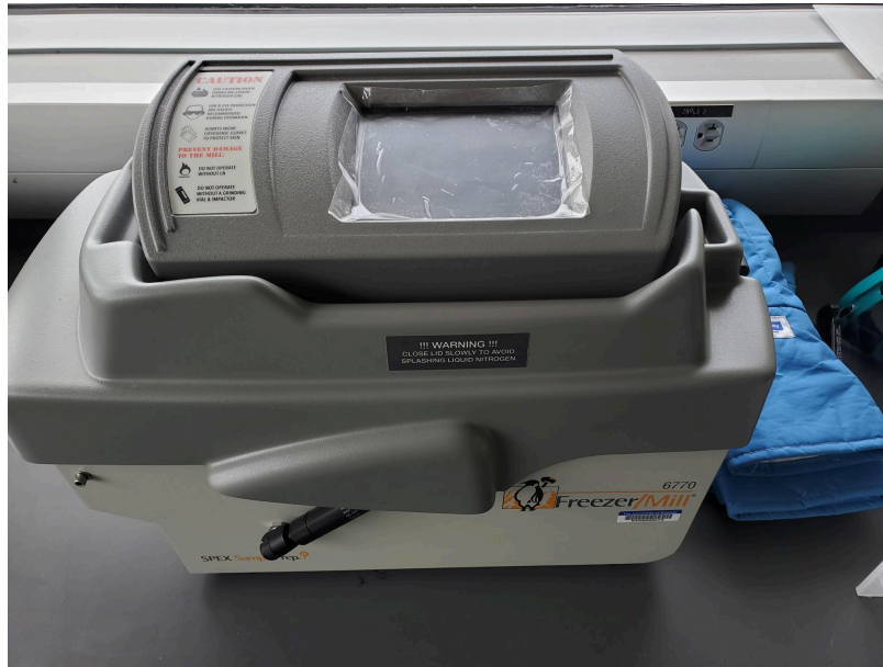
Figure 2.12: SPEX 6770 Cryogenic Mill used with liquid nitrogen to mill \alpha -1,3-glucan-palmitate thermoplastic polysaccharides.
