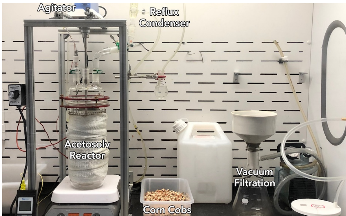
Figure A.6: Photo of acetosolv extraction setup including 4 L reactor with mixer and vacuum filtration.
